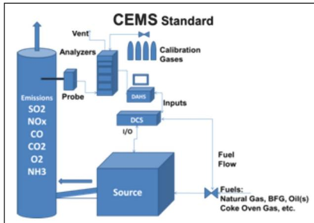
Fig. 1 Standard CEMS Configuration
