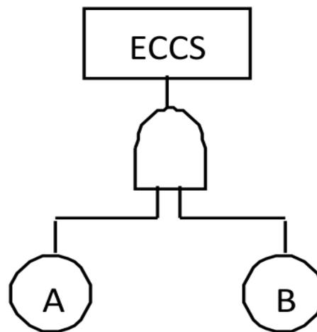
Figure3. Fault Tree of ECCS
