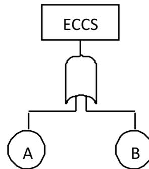
Figure6. Fault Tree of ECCS
