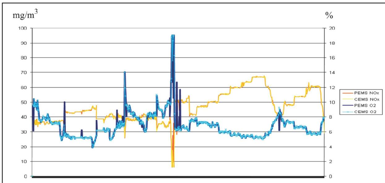
Figure 3 Comparison of PEMS / CEMS results for NOx und O2 (oil-fired boiler).
