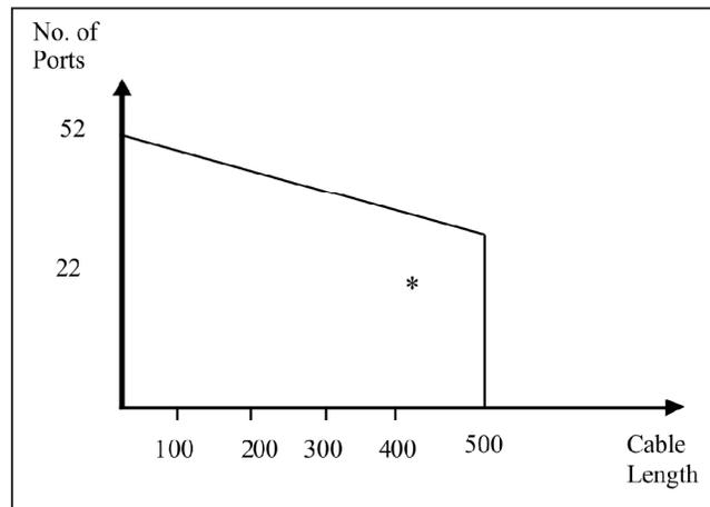
Figure: 2 Relation between no. of nodes and length of LAN cable
