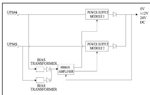
Fig.3 Current Sharing Mode Power Supply
