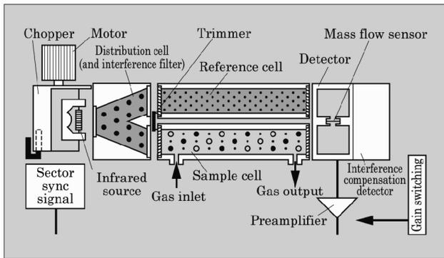
Fig. 2 Configuration of double-beam type measurement unit
