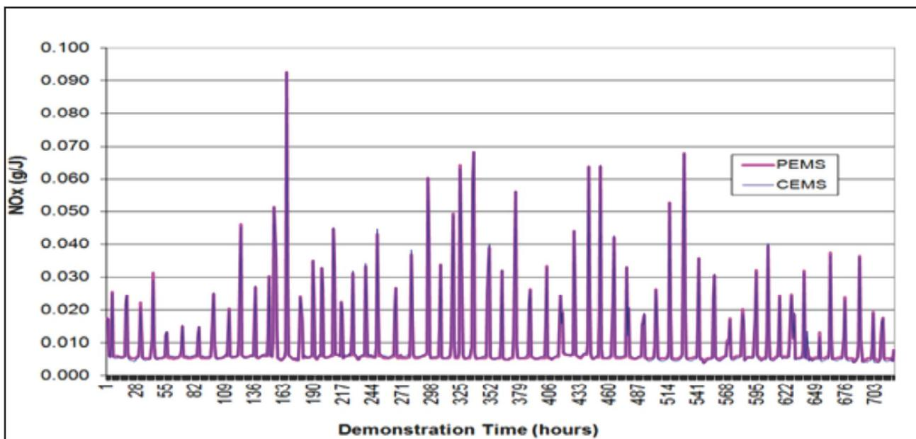
Figure 4 Time plot PEMS versus CEMS for NO<sub>x</sub> emitted by a peaking gas turbine. Comparison period 720 hours (Part 75 certification)
