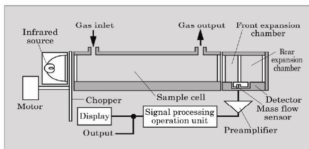
Fig.1 Configuration of single-beam type measurement unit
