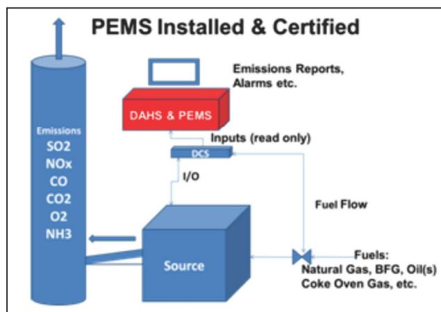
Fig. 2: Emissions Monitoring with PEMS and Data Acquisition (DAHS)
