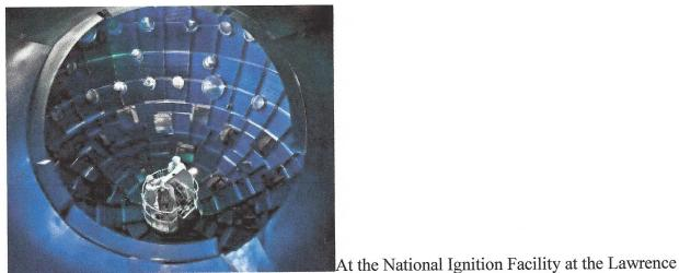
Livermore National Laboratory, in California, scientists are using 192 lasers and 500 trillion watts of power in an attempt to fuse hydrogen, to create miniature stars. These lasers are all focused on a tiny cylinder of beryllium, called a *hohlraum*, that contains a mixture of deuterium and tritium — hydrogen isotopes — and when the switch is thrown, the isotopes are heated to
