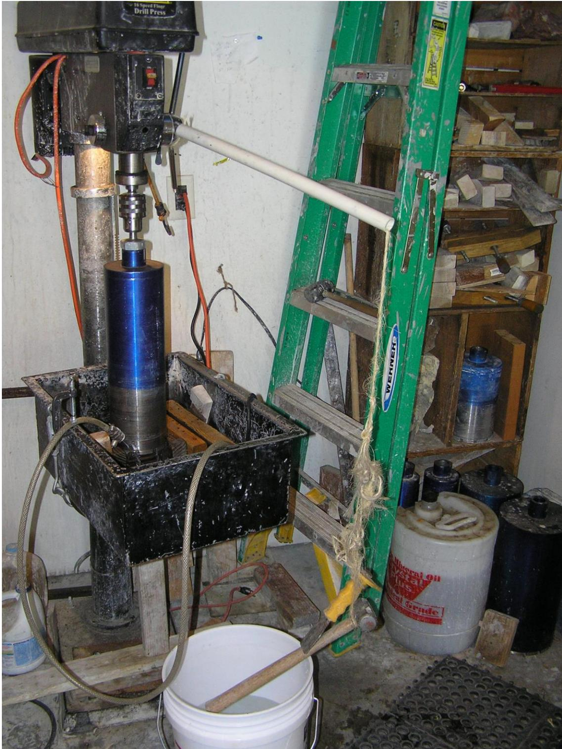
If your rock is more than three inches thick, you will need to raise the drill press work table (with your box, rock and water in it) after a while. Mine has a throw of about 80 millimeters. Do this while the press is running. Loosen the clamp on the riser of the press so that you can crank up the table. Support the table's weight with one hand while
