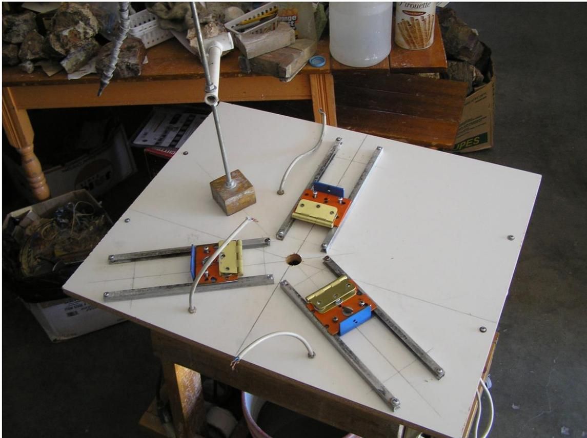
**Wire motors:** Run the power cords through the table surface from below for hookup to the motor wiring. Connect with wire nuts. The other end of the power cord should have a plug attached – yes, a three prong plug. You are working around water and all of your motors should be grounded. The motors should come with a wiring diagram and
