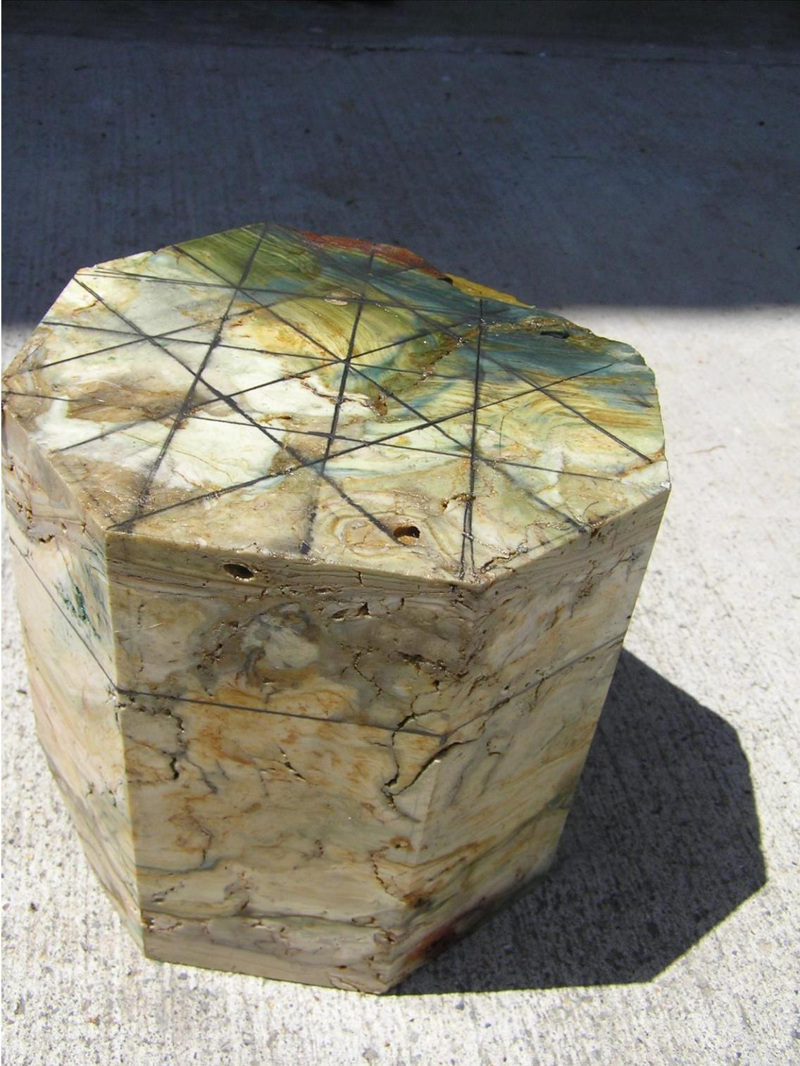
You have now drawn the lines showing where to make the final 16 cuts on your preform. Put it into the saw and make them. To minimize the chances of the preform slipping in the vise and damaging your saw blade, make a wooden support with a v-notch cut out of the bottom to support the weight of the preform. I make every other cut on one end (4
