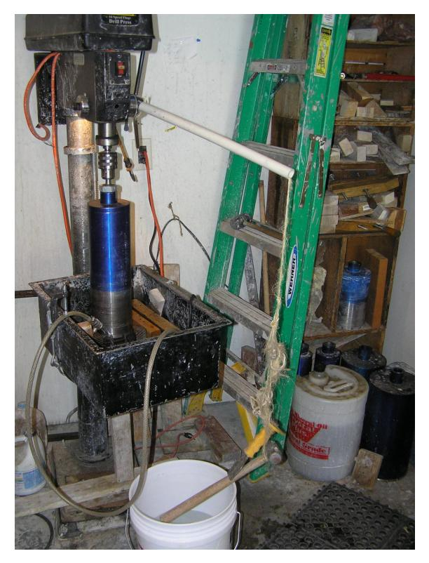
If your rock is more than three inches thick, you will need to raise the drill press work table (with your box, rock and water in it) after a while. Mine has a throw of about 80 millimeters. Do this while the press is running. Loosen the clamp on the riser of the press so that you can crank up the table. Support the table's weight with one hand while
