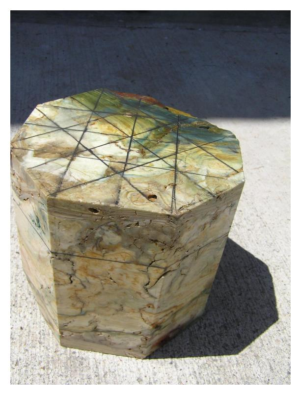
You have now drawn the lines showing where to make the final 16 cuts on your preform. Put it into the saw and make them. To minimize the chances of the preform slipping in the vise and damaging your saw blade, make a wooden support with a v-notch cut out of the bottom to support the weight of the preform. I make every other cut on one end (4
