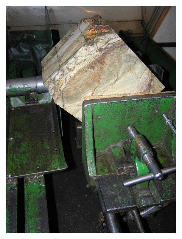
Clean up the rock to get the oil off. Make a mark in the center of each of the eight top edges. Draw lines on the top face connecting marks on opposite edges. There will be four lines and in a perfect cube (seldom happens) they will all intersect in the center of the top face. On each line, measure out from the intersection point the same distance you
