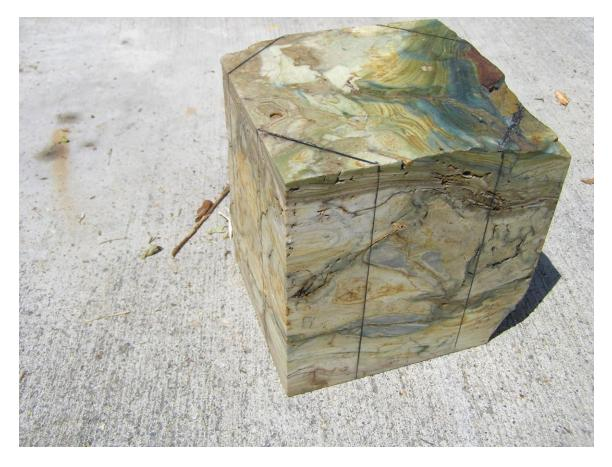
Flip the cube over and do the same thing for the bottom side. Then draw lines on the side faces of the cube connecting the matching marks on each face. Cut the corners off the cube with your rock saw following the lines you have made. You should end up with a solid octagon and four triangular lengths that used to be the corners of the cube.
