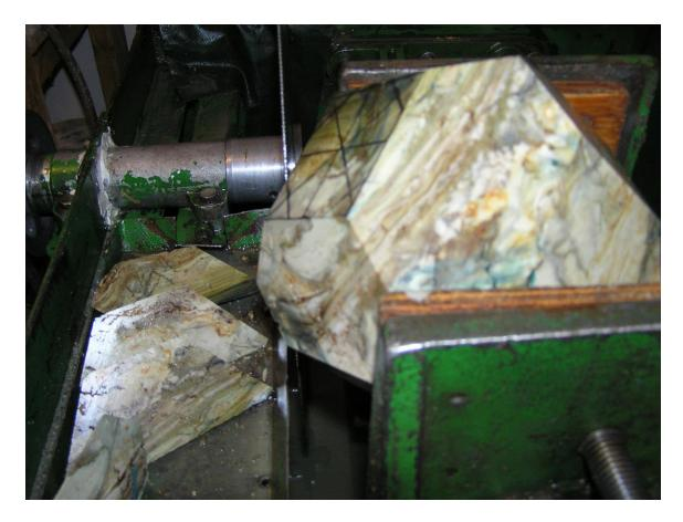
large cuts), flip it over, do the same on the other end (4 more cuts), do the remaining 4 small cuts on that end, then flip it over again and do the last 4 cuts. It will be easier if the second set of four cuts is staggered 45 degrees to the first set because that will give you a flat surface to set the rock on for the last 8 cuts. Trust me. Your preform is now done – knock off some of the corners with a grinder and it is ready to put into the sphere machine.
