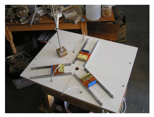
**Wire motors**: Run the power cords through the table surface from below for hookup to the motor wiring. Connect with wire nuts. The other end of the power cord should have a plug attached – yes, a <u>three prong plug</u>. You are working around water and all of your motors should be grounded. The motors should come with a wiring diagram and
