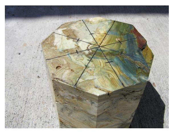
Next turn the rock on its side, measure inward from one of the ends along an edge a distance equal to  $\frac{1}{2}$  the diameter of the rock times 0.58 minus 1 millimeter. Make a mark with your pencil at this point. Repeat for the other seven edges, then connect all of these marks together with lines. Turn rock around and repeat for the other end.
