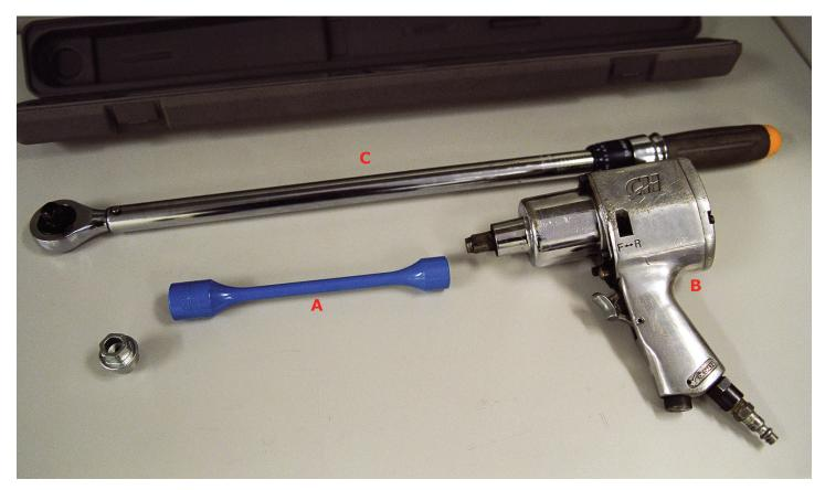
Figure 8. A: an 80 foot-pound Torq Stik. B: air wrench that Torq Stik attaches to. C: A manual torque wrench.
