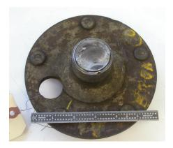
**Figure 2.** The end of a Ford Bronco axle broke off one month after it was serviced. During the service an axle bearing was carelessly removed with a cutting torch, which metallurgically altered the axle and led to a catastrophic fatigue fracture.
