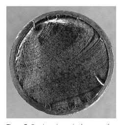
**Figure 7.** Beach marks on the fracture surface are clear signs that this stud from the right rear of a van failed from fatigue. Failure was less than 121 days since installation.
