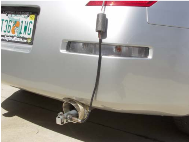
Figure 3 – Exhaust Sniffer Vehicle Installation
