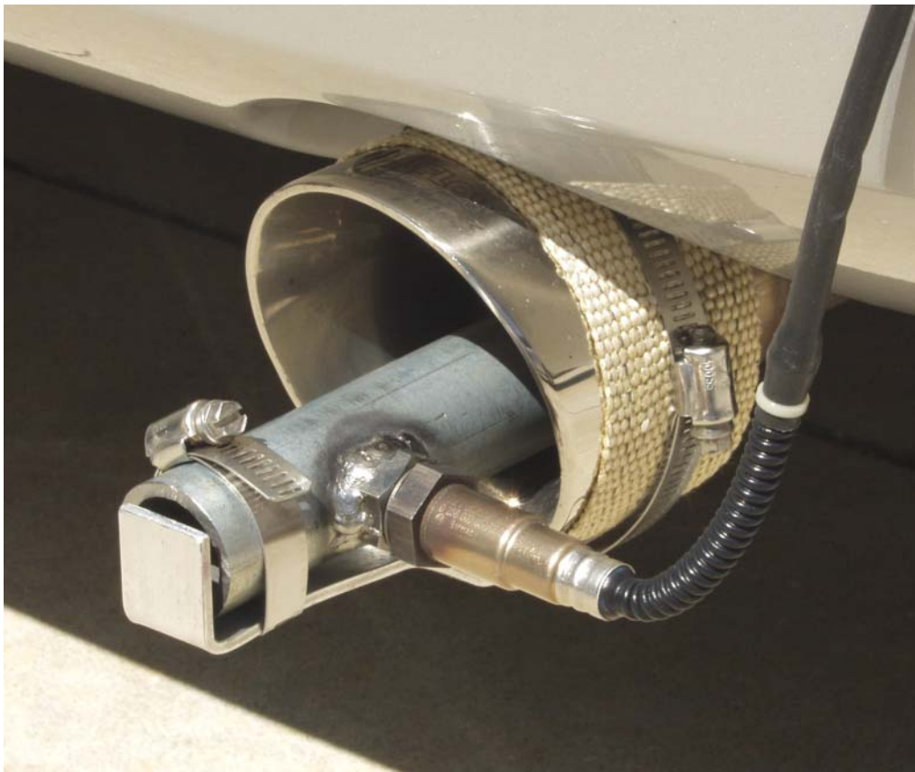
Figure 2 – Exhaust Sniffer Vehicle Installation
