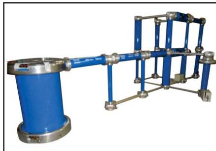
280kV, Impulse Voltage - Test Set-up
