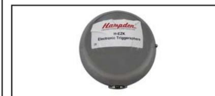
Electronic Trigger Sphere used for controlled triggering of Impulse Generator. It has the same dia. as that of passive spheres(100mm) used in Sphere-gap (KF) enabling easy interchange. The trigger energy is supplied by battery operated electronic circuit inside the Trigger-Sphere. The command pulse from Trigger Unit (TU) is fed via Fiber-optic Cable.
