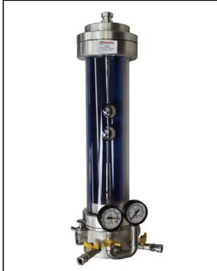
For the determination of flashover voltage of different electrode configurations as a function of vacuum and pressure
