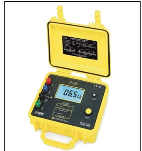
Earth Ground Tester, Earth Ground Resistance Range 0 to 2000k Ohms, Resolution 0.01 to 1 Ohms, Operating Frequency 128 Hz, Accuracy +/-2 Percent of Reading +/-1 Count, Measuring Current 0.1 to 10mA Earth Volts 42VAC, Soil Resistivity Yes, Display Digital LCD, Counts 1999, Power Source (8) C Batteries, Alkaline Recommended, Standards IEC, CE, EN 61010-1, Pollution Degree 2, Safety Rating CAT III 30V Includes (8) C Batteries and Instructions.
