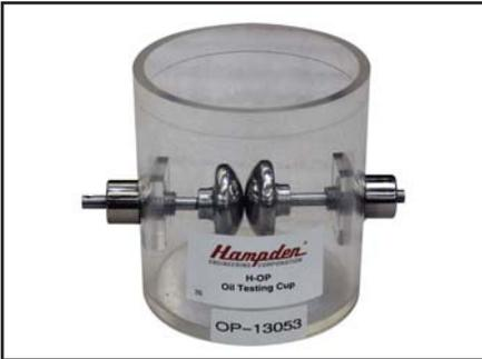
With electrodes having spherical shape with a gap-setting of 2.5mm
