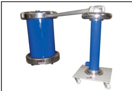
11kV, AC Voltage - Test Set-up
