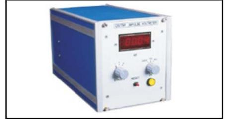
For measurement of High Voltage Impulse with Digital Display Provision for external Oscilloscope waveform display. To be used in conjunction With Impulse Divider (CB) and LV Divider (NTZ), 10m measuring-cable and housing.
