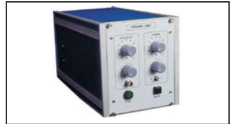
The Electronic Trigger Unit (TU) in conjunction with Trigger Sphere (EZK) is used to fire the sphere-gap(KF) or chopping output voltage using Measuring Spark gap (MF100). This ensures reproducible test results and Oscillograms
