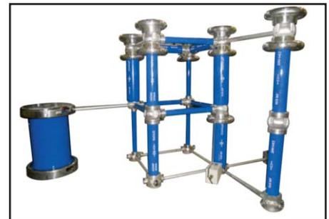
280kV, DC Voltage Test Set-up
