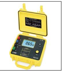
Earth Ground Tester, Earth Ground Resistance Range 0 to 2000k Ohms, Resolution 0.01 to 1 Ohms, Operating Frequency 128 Hz, Accuracy +/-2 Percent of Reading +/-1 Count, Measuring Current 0.1 to 10mAEarth Volts 42VAC, Soil Resistivity Yes, Display Digital LCD, Counts 1999, Power Source (8) C Batteries, Alkaline Recommended, Standards IEC, CE, EN 61010-1, Pollution Degree 2, Safety Rating CAT III 30VIncludes (8) C Batteries and Instructions.
