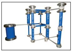
280kV, DC Voltage Test Set-up
