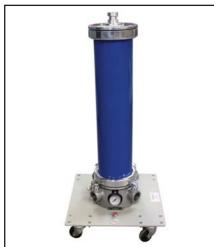
SF6 insulated Compressed Gas Standard capacitor in FRP housing Mounted on mobile platform and with Coronafree HV Electrode RATED VOLTAGE = 100kV, 50/60Hz RATED TEST VOLTAGE = 110 kV RATED CAPACITANCE = approx. 37pF +/-10% SF6 Compressed gas Standard Capacitor, Tan delta=.002% Filling Pressure (abs) = 3.5bar Coupling Capacitor (H-CK120):
