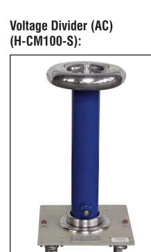
Oil insulated and hermetically sealed capacitor in FRP housing Mounted on mobile platform and with Coronafree HV Electrodes RATED VOLTAGE = 300kV, 50/60Hz RATED TEST VOLTAGE = 360kV, 50/60Hz RATED CAPACITANCE = 100pF + / -10%RATED PD LEVEL < 5pC
