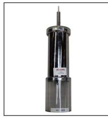
For determination of glow intensity as a function of wire diameter. The corona cage has to be inserted into the WSTS Vessel for vacuum and pressure (type DKU). The measurement can be made at vacuum and also at higher pressures. Vessel for Vacuum and Pressure with Suitable Pump & Compressor (H-DKU):
