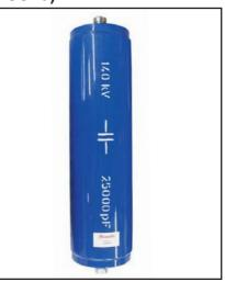
Oil impregnated and PU resin cast impulse Capacitor RATED VOLTAGE = 140kV, dc RATED TEST VOLTAGE = 160kV, dc RATED CAPACITANCE = 25nF +/-10%
