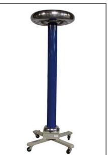
Oil insulated and hermetically sealed capacitor in FRP housing Mounted on mobile platform and with Coronafree HV Electrodes RATED VOLTAGE = 300kV, 50/60Hz RATED TEST VOLTAGE = 360kV, 50/60Hz RATED CAPACITANCE = 1000pF +/-10% RATED PD LEVEL < 5pC
