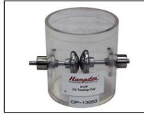
With electrodes having spherical shape with a gap-setting of 2.5mm Used for the measurement of breakdown voltage
