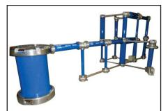
280kV, Impulse Voltage - Test Set-up
