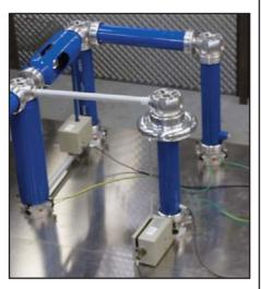
Earthing Switch H-ES in use. Control Desk control triggers rod.
