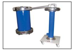
11kV, AC Voltage - Test Set-up
