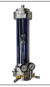
For the determination of flashover voltage of different electrode configurations as a function of vacuum and pressure
