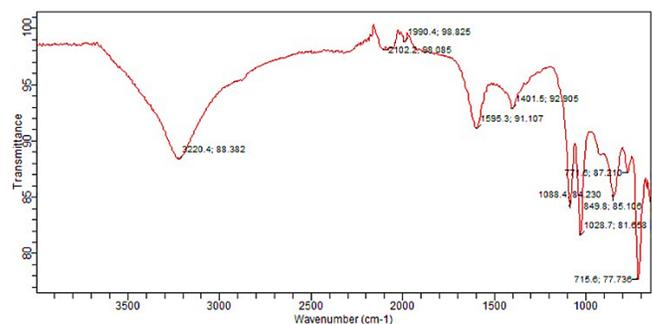
**Figure 4.** FT-IR absorption spectra of copper oxide nanoparticles.
