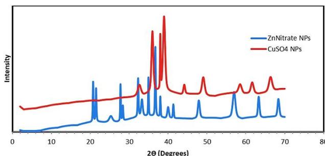
**Figure 7.** XRD Analysis of Both Zinc oxide and Copper oxide nanoparticles
