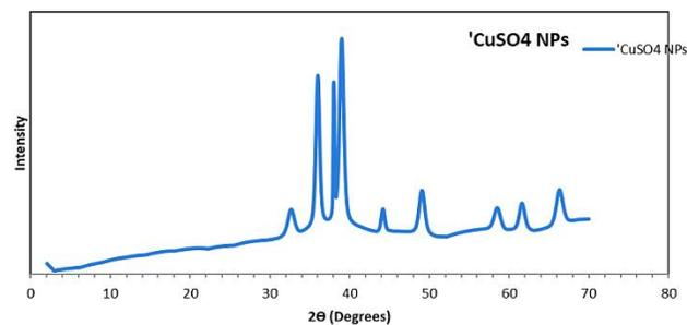
**Figure 5.** XRD analysis of Copper oxide nanoparticle
