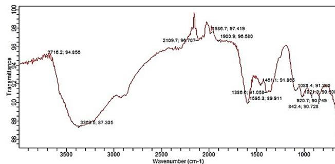
**Figure 3.** FT-IR absorption spectra of zinc oxide nanoparticles.
