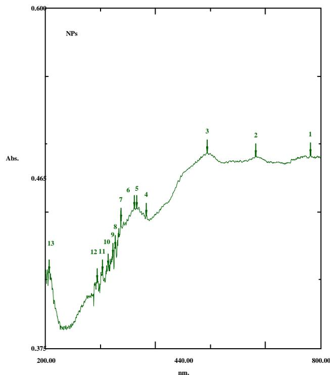
Figure 1. The UV-visible absorption spectrum of zinc oxide nanoparticles synthesized from *Azadirachta indica* (Neem) Bark extract.
