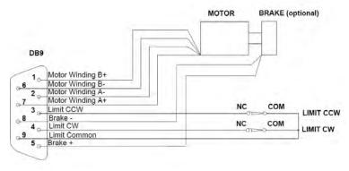
ADC uses a standard male DB-9 Connector for both the motor and limit switches.
