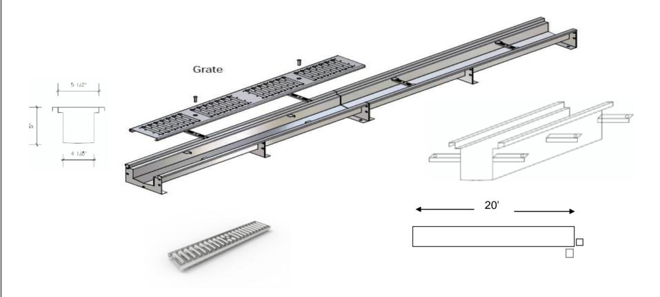
**Engineering Specification:** 6" Wide 14 Ga. 304 Stainless Steel Trench Drain System; Fully Welded End Caps; Outlets; Joints In Factory; Stainless Slotted; ADA Class "A" Non-Traffic Grate.
