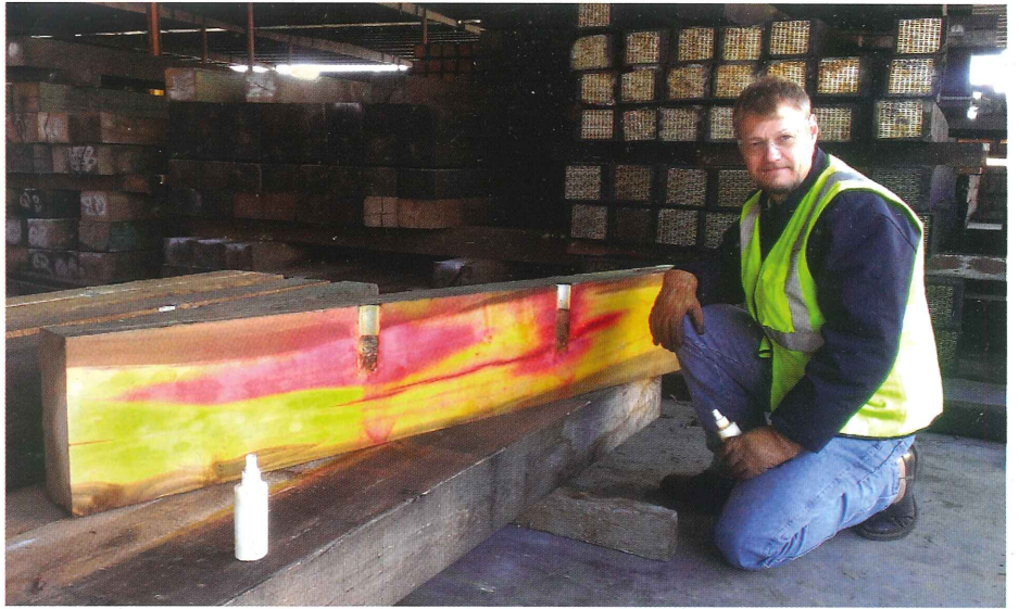
Dr. Jeff Lloyd kneels next to a bridge timber that was cut in half, sectioned longitudinally, and sprayed with curcumin to show the borate penetration (red areas) immediately after treatment. Also note the vertical BTX ports that were used to inject the borates at initial treatment.
