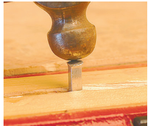
(Top) While holding the salt mill upside down, the adjusting knob pressed against the head and the grinder core fully in the housing, mark the shaft flush with the bottom of the grinder core.(Bottom) Cut off the extra material and peen the end over so it looks like the factory-prepared end cut off earlier.
