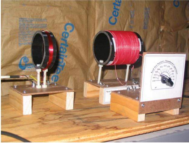
Figure 1: Q Measurement Bench Setup
