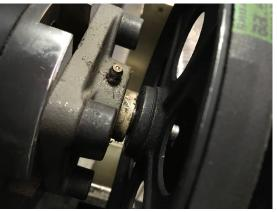
In the event a back bearing should start to go bad it will likely begin to make noise. Perhaps a rubbing or squeaking sound. This requires attention before entire bearing goes bad which could lock up drum. On the 2016 and earlier Sedona 3200 (not the DW model) you will need to remove the 4 bolts in the electric room to move it to the side to reach bearing and pulley.
