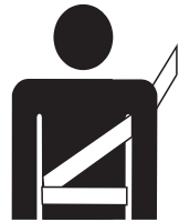
The wrong way to wear a safety belt.
