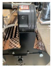
**3. N**EXT REMOVE TOP BOLT IN NECK OF ROASTER AND REPLACE WITH AIR LINE CONNECTOR
