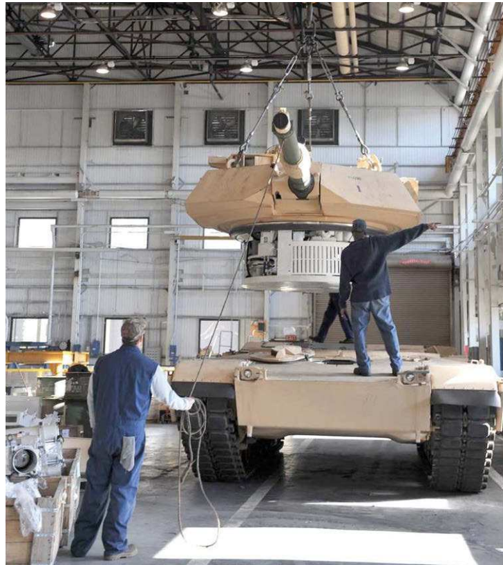
Workers put a turret on a refurbished Abrams tank at JSMC. The Army intends to use upgraded variants of the tank until at least 2050, but its orders have been filled, and the current tank fleet meets specifications. Meanwhile, since 2011, the plant has produced hundreds of the Army’s IED-defensive Stryker DVH, of which more than 450 have been used in Afghanistan. General Dynamics
