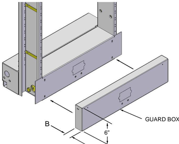
**UEF Guard Boxes** install on the side of the rack opposite of the guard rail. These allow for custom tailoring the footprint of the equipment rack. These guard boxes feature an electrical cutout for AC convenience outlets. AC covers sold separately.
