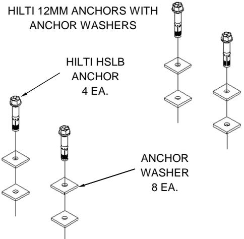
**FOR USE IN SEISMIC INSTALLATIONS WITH CC&R UEF OR NETWORK RACKS**
