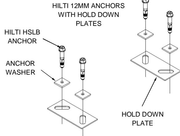
**FOR USE IN SEISMIC INSTALLATIONS WITH DIAGONAL ANCHOR SLOTS**
