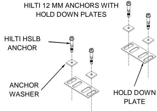
**FOR USE IN SEISMIC INSTALLATIONS WITH CC&R UEF OR NETWORK RACKS**
