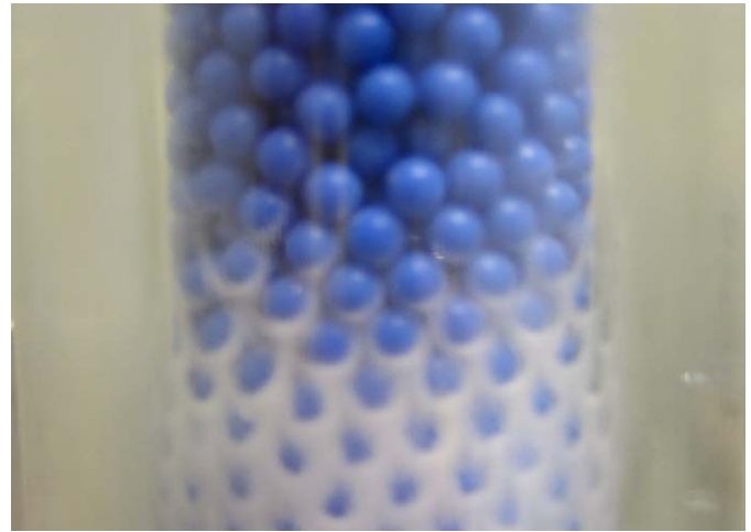
Fig. 4. CO_2 ice formed at the packing surface during a capture cycle.
