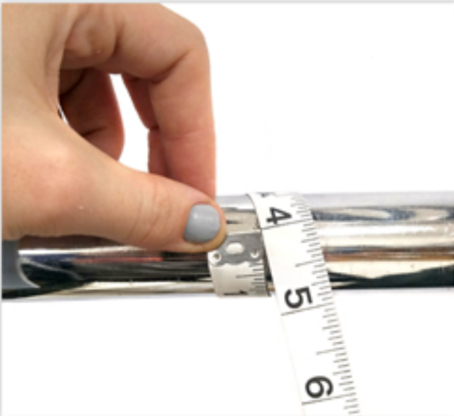
Pipe or Z Rack: Approximately 4" in circumference
