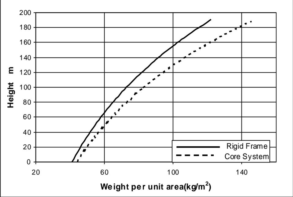
**Figure (8):** Relationship between height and material weight per unit area
