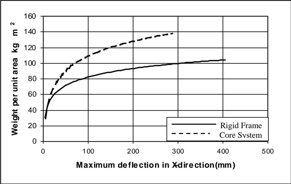
**Figure (9):** Relationship between material used and deflection in X-direction
