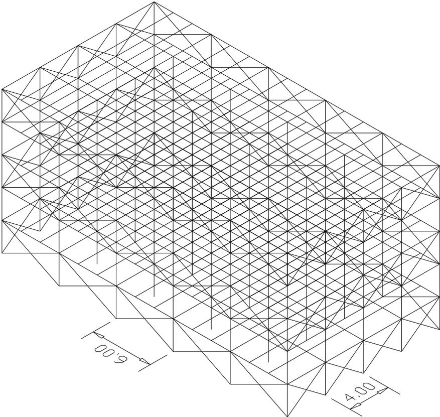
**Figure (5):** Lateral load resistance using exterior truss system
