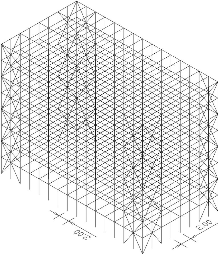
**Figure (4):** Lateral load resistance using tube system
