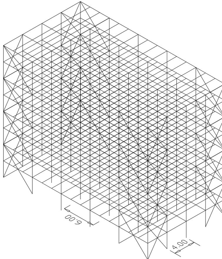
**Figure (3):** Lateral load resistance using rigid framing system
