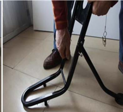
2. Install legs with 5/16x1-1/4 bolts and 5/16 Nuts.
