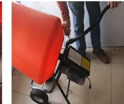
9. Install handles and clevis pin with land yard.
