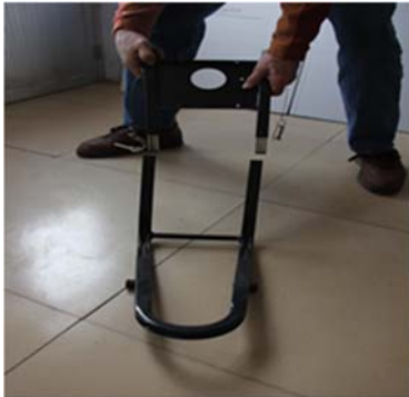
1. Put together upper and lower main frame. Do not Put in bolts.
