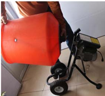
7. Slide on drum. Line up 1/2" hole.
