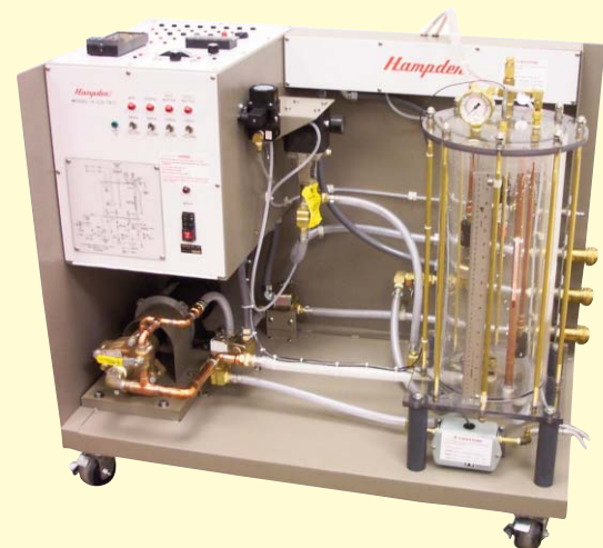
MODEL H-ICS-7617 Instrument and Process Control Trainer
