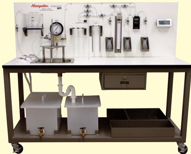
MODEL H-6535 Hydrostatics Bench
