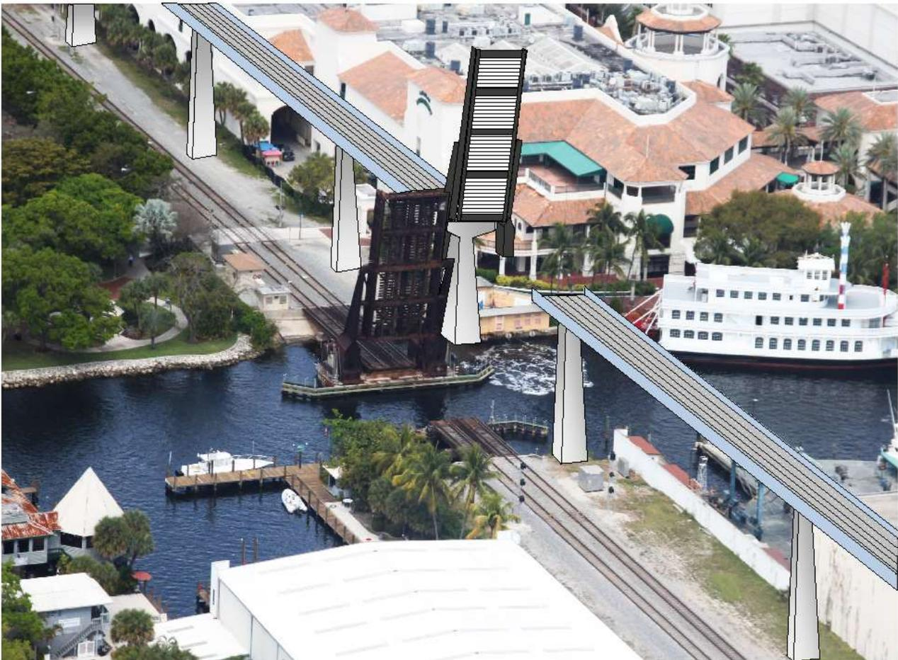
**CONCEPTUAL RENDERING OF HIGH LEVEL MOVABLE PASSENGER RAIL BRIDGE AND VIADUCT OVER THE NEW RIVER**
