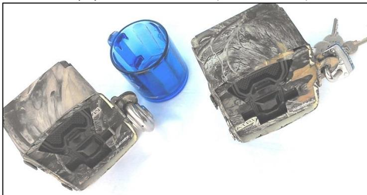
of the bridges. (See photo inset showing cameras and other objects for scale.) Security boxes were fabricated to fit each camera, and they were mounted to a piling on private property to obtain a close view of the boats navigating and the bridge opening and closures. The camera installed facing the CSX bridge was further away from the bridge than the camera mounted near the FEC bridge. Each camera was tested for time lapse and motion
