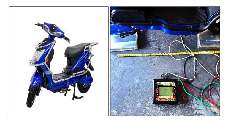
This vehicle also is street legal and had brakes lights, directionals, rear view mirrors, and crash bars all around. Its range is approx. 20-25 miles with a 60V/20Ah Lead-acid battery,
