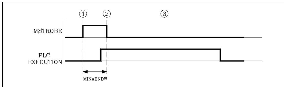
2. The CNC will keep the general logic output "MSTROBE" active during the time indicated by means of g.m.p. MINAENDW (P30).
