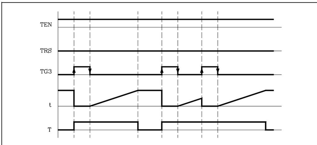
If, once the timing has finished, it is required to activate the timer again, another leading edge must be produced at the TG3 input.
