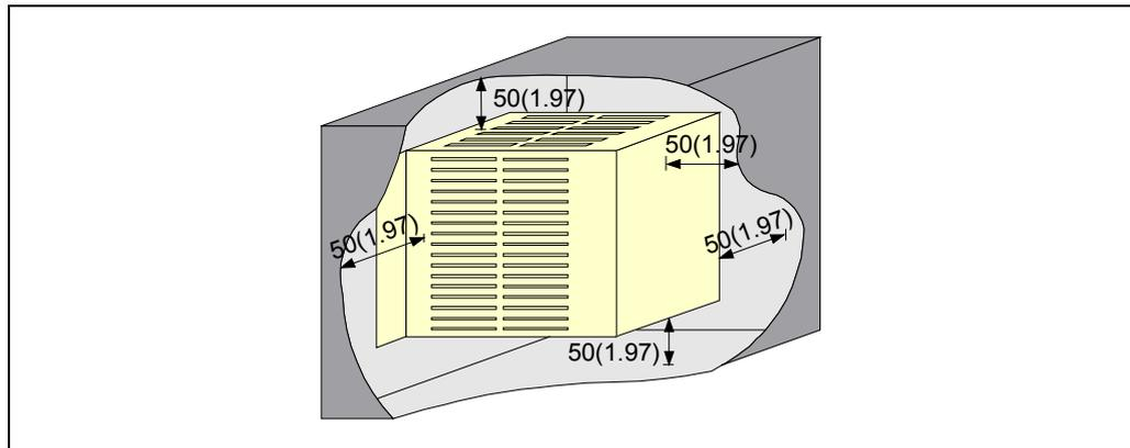
When using a fan to better ventilate the enclosure, a DC FAN must be used since an AC fan may generate electromagnetic interference resulting in distorted images being displayed by the CRT.
