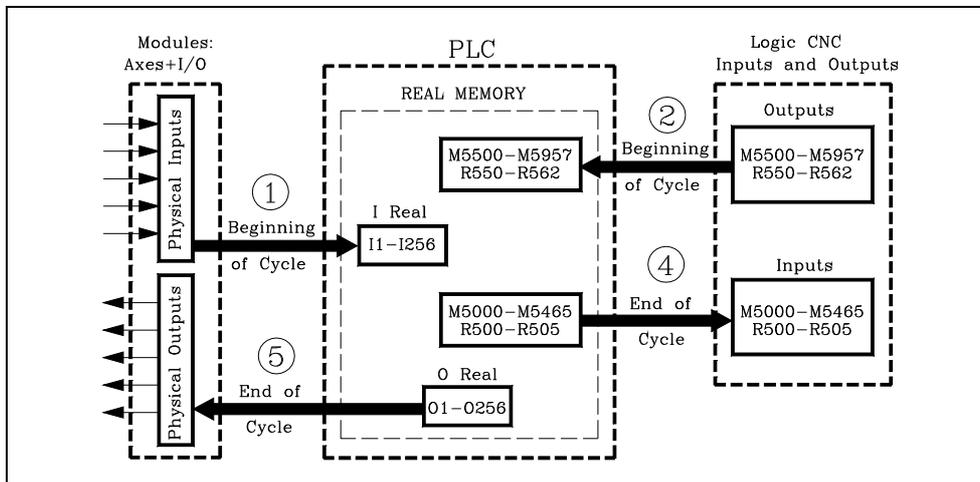
2. It allocates the current values of the logic CNC outputs (CNCREADY, START, FHOUT, etc.) to PLC resources M5500 thru M5957 and R550 thru R562 .
