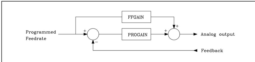
For example, if a.m.p. FFGAIN (P25) has been set to "80", the axis velocity command will be:
