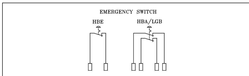
The HBE handwheel has one contact and the HBA and LGB models have a dual safety contact.
