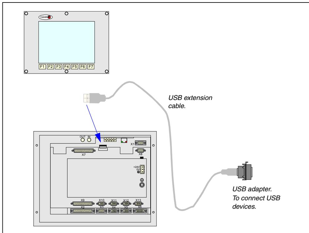
3. Once the extension set has been properly connected, it will be possible to connect and disconnect USB devices to the CNC while it is on.
