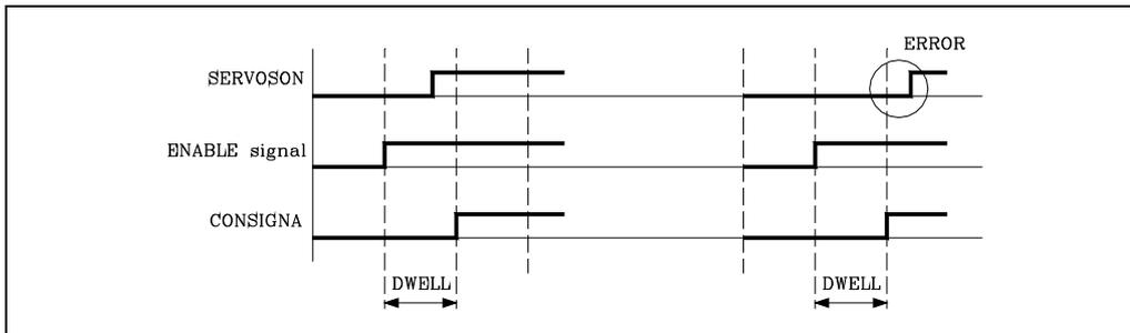
Also, if it changes to low during the rotation of the spindle, the CNC will stop the axes feed and the spindle rotation displaying the corresponding error message.
