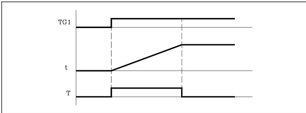
If the timer is initialized with values TEN=1 and TRS=0, the timer will be activated when a leading edge is produced at input TG1. At that moment, the timer status output (T) changes states (T=1) and the timing starts from "0".
