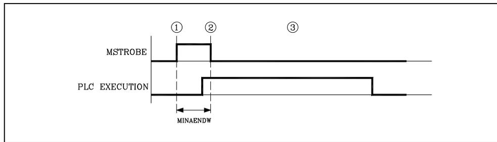
2. The CNC will keep the general logic output "MSTROBE" active during the time indicated by means of g.m.p. MINAENDW (P30).
