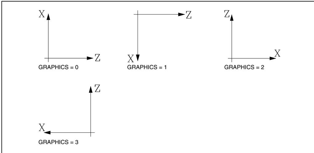
On M, MC, and MCO models, this parameter indicates the axis system being used for the graphic representation as well as the motion possibilities for the W axis added to those of the Z axis in the graphic representation (W additive).
