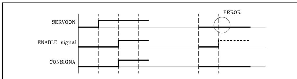
If the SERVOON signal is high, the CNC allows the movement of this axis by activating the ENABLE signal and providing the required velocity command output.
