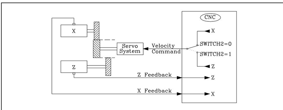
The two axes share the same feedback device. It must be connected to the feedback connector of the main axis.
