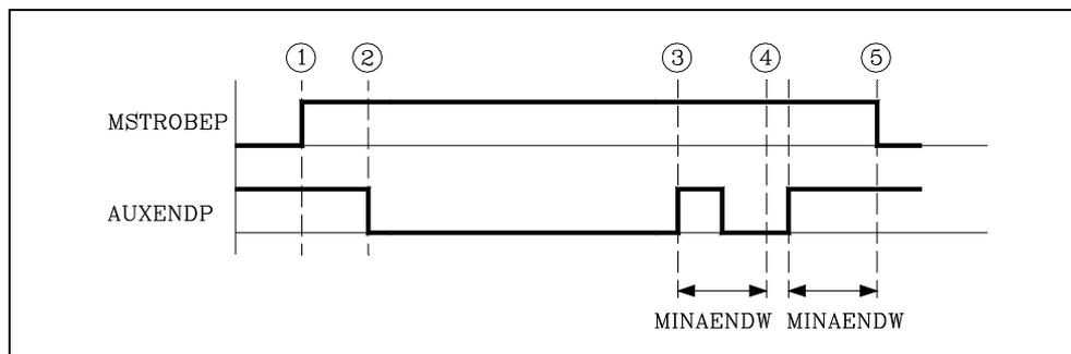
2. When the PLC detects the activation of the "MSTROBEP" signal it must deactivate the general logic input "AUXENDP" to "tell" the CNC that the execution of the function has started.
