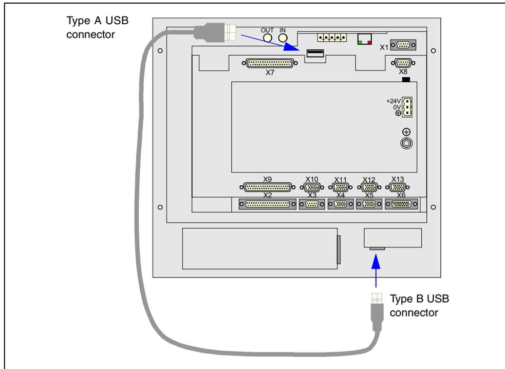
2. Once the extension cable is connected, it will be possible to use the USB connector of the front of the keyboard, while the CNC is on.
