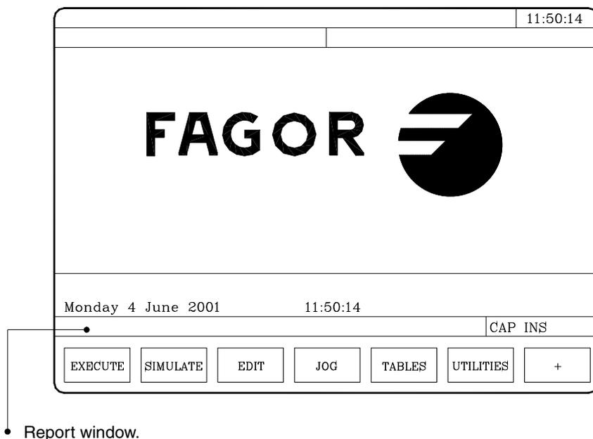
The CNC allows the display of a previously defined screen instead of the Fagor logo. Refer to the operating manual.
