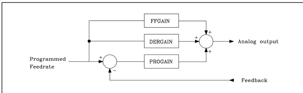
Best results are usually obtained when using it as AC-forward Gain, "ACFGAIN" (P42) = YES together with feed-forward gain.
