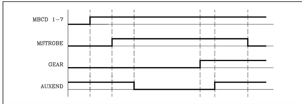
Once the general "AUXEND" input is activated, the CNC will require that this signal be kept active for a time period greater than the value given to the g.m.p. MINAENDW (P30).
