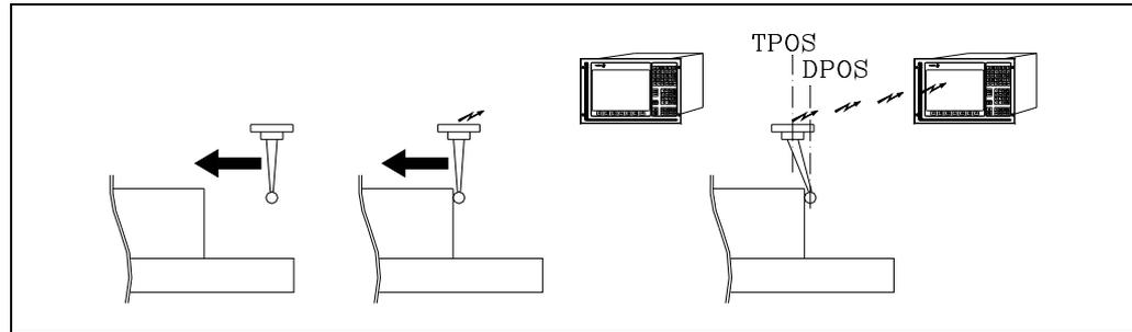
The probe keeps moving until the CNC receives the probe signal.
