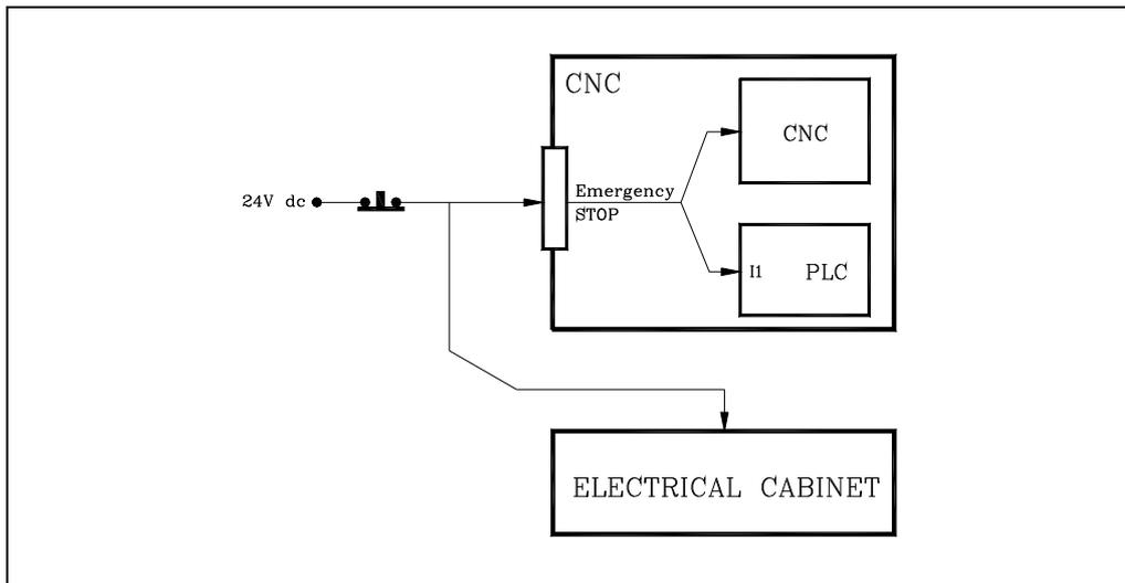
During the initializing process carried out by the CNC on power-up, the EMERGENCY OUTPUT of the CNC (pin 2 of connector X10) remains at low (at "0") in order to avoid a premature activation of the electrical cabinet.
