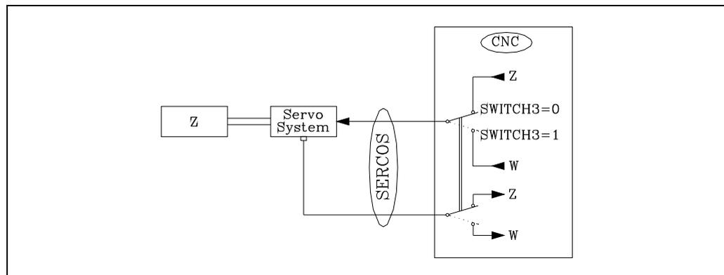
a.m.p. SWINBACK (P66) of the secondary axis must be set to "0".
