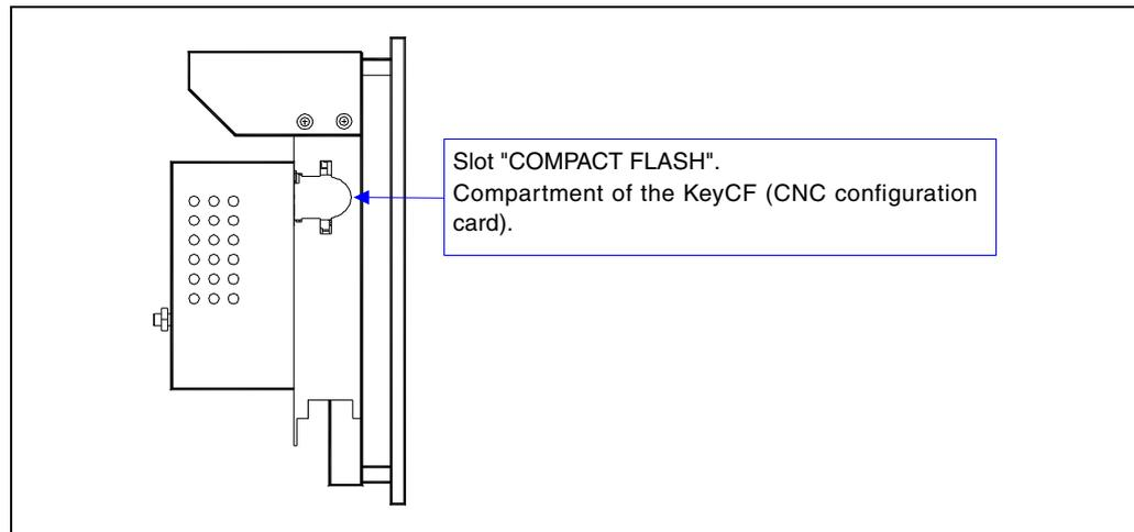
The KeyCF supplied by Fagor with each CNC has an identification code corresponding to:
