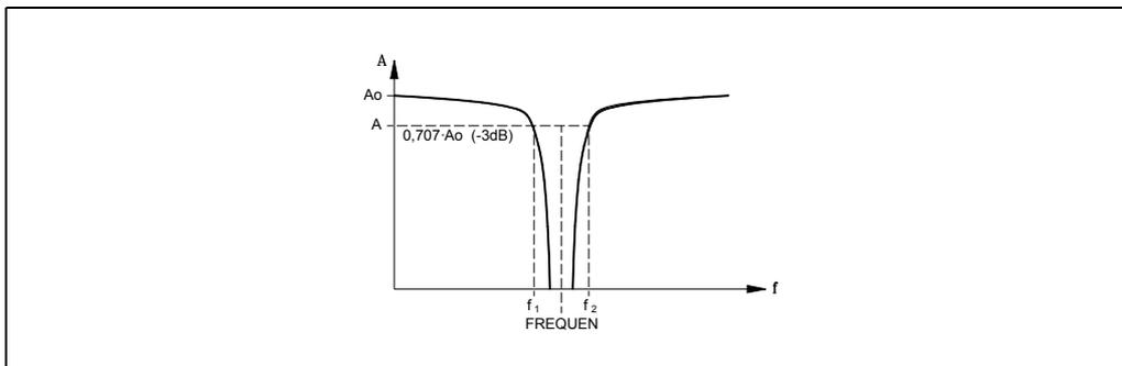
**CNC start-up with Fagor filters active.**
