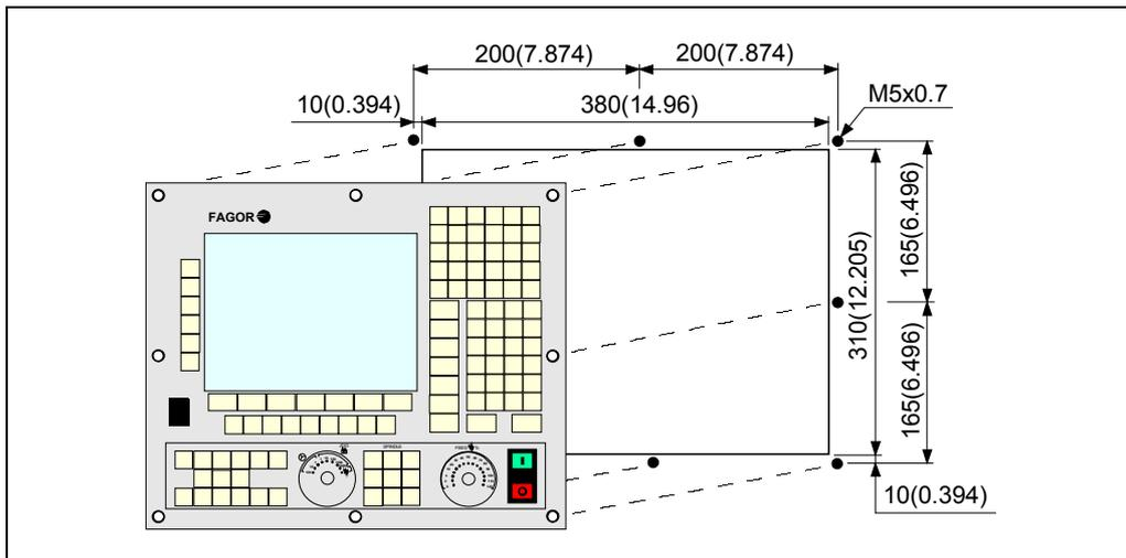
The minimum distance from each side of the monitor to its enclosure in order to guarantee the required ambient conditions is shown below:
