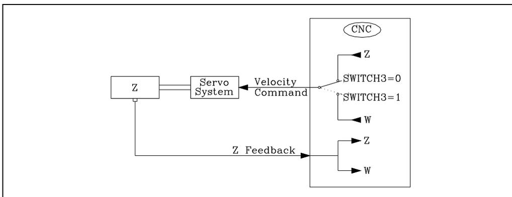
Connect the Z axis feedback (main axis).
