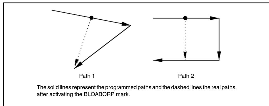
If a block is aborted and then the RETRACE function is activated, the retraced path (backwards) will not be the same as the one traveled forward. The two paths will not coincide either when aborting a block while the RETRACE function is active.
