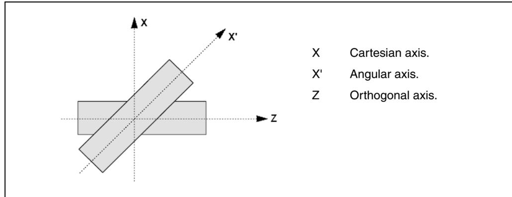
Programming in the Cartesian system (Z-X) requires activating an angular transformation of an inclined plane that converts the movements of the real (non-perpendicular) axes (Z-X'). This way, a movement programmed on the X axis is transformed into movements on the Z-X' axes; i.e. it then moves along the Z axis and the angular X' axis.
