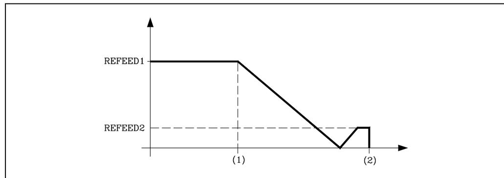
When the selected axis does not have a machine reference (home) switch (a.m.p. DECINPUT (P31) = NO), the CNC will move the spindle at the feedrate set by a.m.p. REFEED2 (P35) until the first marker pulse from the current position is found, thus ending the home search.
