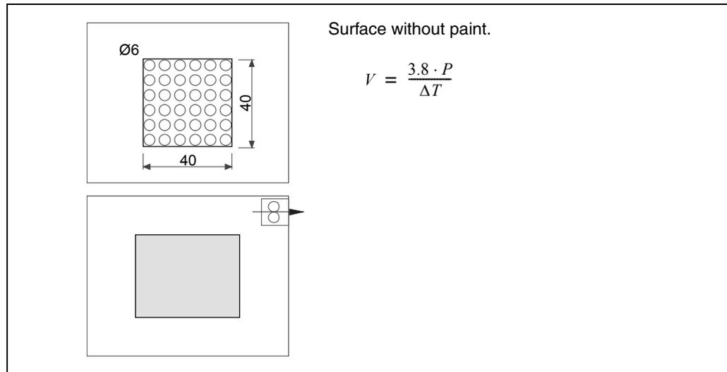
Bear in mind that this air flow through the unit extracts hot air to the outside, but it allows dirt into the enclosure. Thus, a filter should be installed to maintain the ambient conditions allowed.
