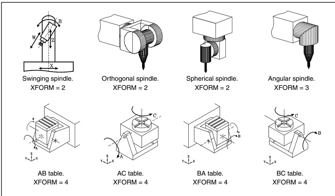
**Definition of the kinematics of a swinging, orthogonal or spherical spindle (XFORM = 2)**
