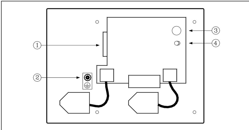
1. SUB-D type 25-pin female connector to connect the keyboard with the central unit or with a switching board.
