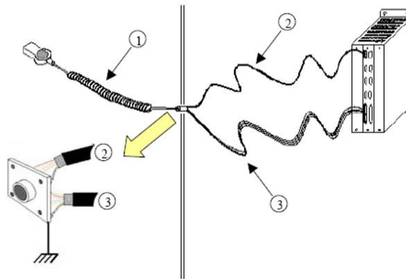
With the 8055 CNC, use a 7x1x0.14 PVC shielded cable for the feedback cable (2) of 5 V. The shield of both cables must be connected to the connector and to ground.
