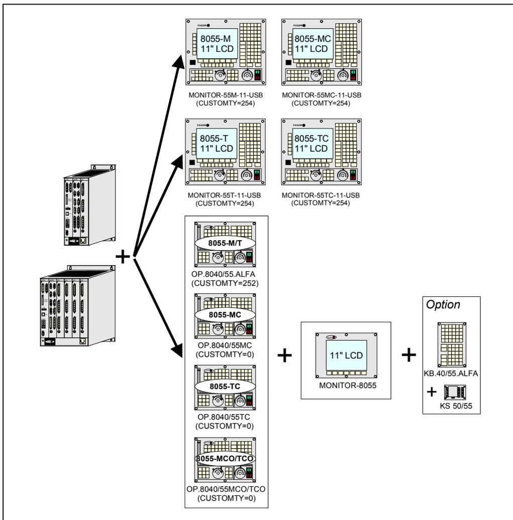
Use the video signal cable (up to 40 m) to connect the monitor with the central unit and the keyboard signal cable (up to 25 m) to connect the keyboard with the central unit.
