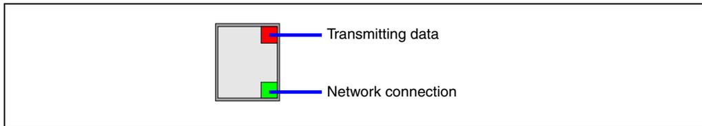
The Ethernet option permits configuring the CNC as another node within the local area network. This makes it possible to communicate with other PC's to transfer files or carrying out telediagnostic tasks.
