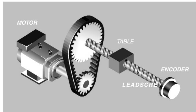
We have an axis with a maximum feedrate of 20 m/min, with a leadscrew pitch of 20 and a 3-to-1 gear ratio between the motor and the leadscrew. The encoder is an HOP model (Vpp) and provides 18,000 pulses per turn. If a linear encoder is a FAGOR GOX model with a glass/steel-tape grading pitch of 20 $\mu$  and the actual TTL pitch is 4 $\mu$ .
