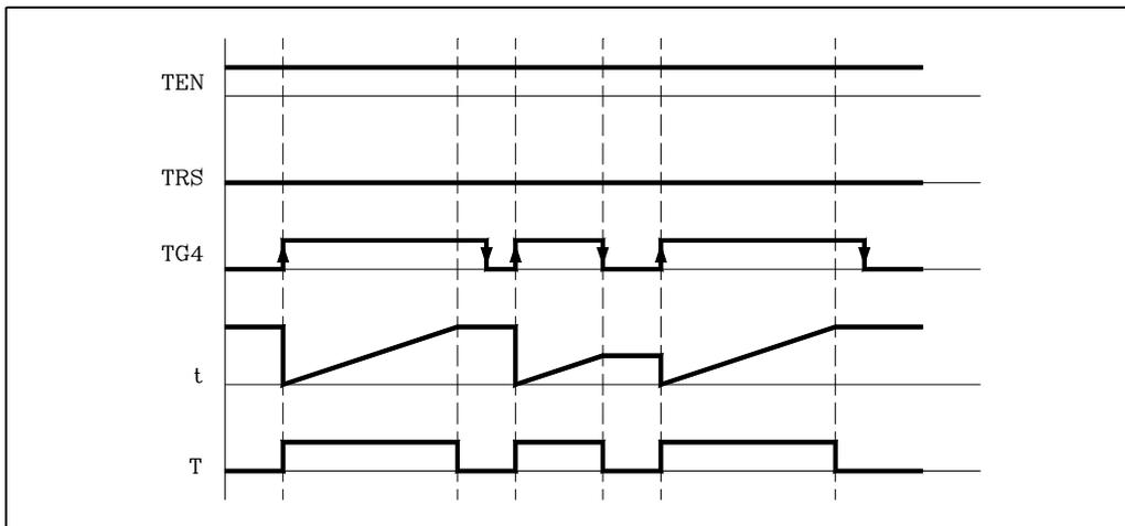
Once the time specified by the time constant has elapsed, timing will be considered as having finished. The time status output (T) changes status ( $T=0$ ) and the elapsed time will be kept as a timer time value (T).
