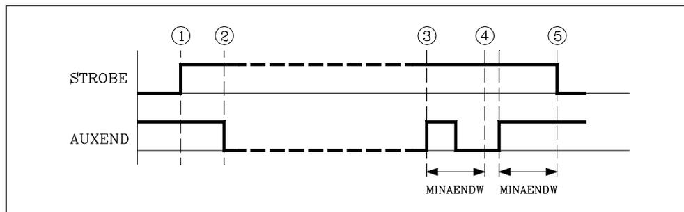
2. When the PLC detects that one of the STROBE signals is active, it must deactivate the general logic input "AUXEND" to tell the CNC that the execution of the corresponding function or functions is starting.
