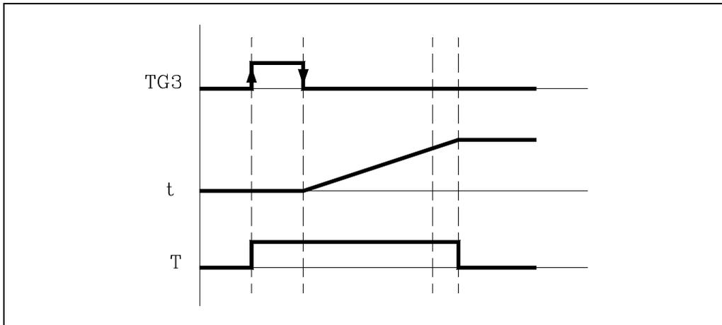
If the timer is initialized with values  $TEN=1$  and  $TRS=0$ , the timer will be activated when a leading edge is produced at the TG3 input. At that moment, the timer status output will have a value of  $T=1$ .
