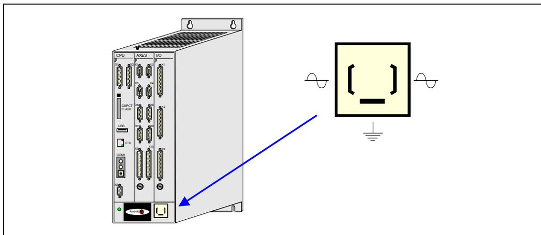
To prevent electrical shock at the monitor of the 8055 CNC, use the proper mains AC connector (A) with 3-wire power cables (one of them for ground connection).
