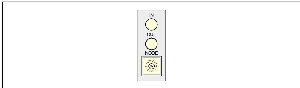
Each element integrated into the Sercos bus is identified with the 16-position rotary switch (0-15) "Address" (also known as Node\_Select). This rotary switch selects the address (node) occupied by each element integrated in the bus.
