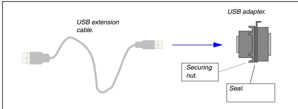
2. While the CNC is off, connect the extension cable to the USB connector of the CNC.
