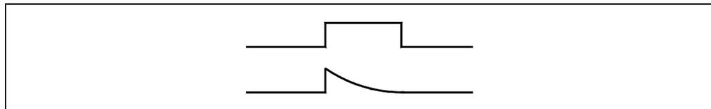
If the duration of the rectangular pulse is adjusted for low speed, it may be too high for high speed or not enough for low speed when adjusted for high speed. In this cases, it is recommended to use the exponential type that applies a strong pulse at the beginning and decreases in time.
