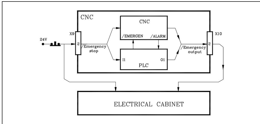
There are two ways to cause an emergency at the CNC, by activating the physical input /EMERGENCY STOP or the general logic input "/EMERGENCY" from the PLC.
