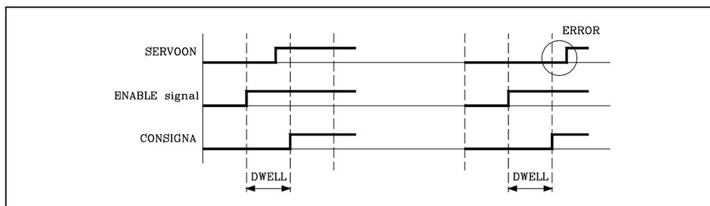
Also, if the SERVOON signal changes states during the movement of the axis, the CNC stops the axes feed and the spindle rotation displaying the corresponding error message.
