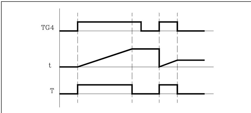
If the timer is initialized with values  $TEN=1$  and  $TRS=0$ , the timer will be activated when a leading edge is produced at the TG4 input. At that moment, the timer status output (T) changes states ( $T=1$ ) and the timing starts from "0".
