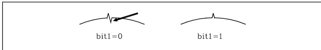
In these conditions, the CNC eliminates the additional command peak in the second position loop after detecting that the moving direction has changed. If the internal peaks are not eliminated, adjust the leadscrew backlash compensation better.
