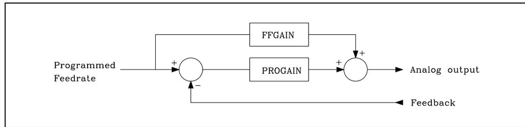
When it is due to variations of the programmed feedrate, "ACFGAIN" (P46) = YES, it is called AC-forward gain" since it is due to acc./dec.
