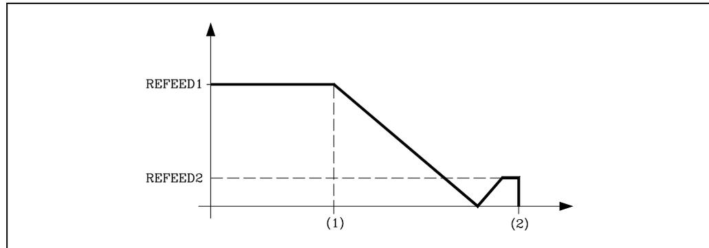
When the spindle does not have a machine reference (home) switch (s.m.p. DECINPUT (P31) = NO), the CNC will move the spindle at the feedrate set by s.m.p. REFEEED2 (P35) until the first marker pulse from the current position is found, thus ending the home search.
