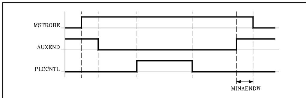
After analyzing the block and detecting the gear change the CNC indicates this to the PLC in one of the "MBCD1-7" registers (M41 to M44) and will activate the general logic output "MSTROBE" to tell the PLC that it must execute it.
