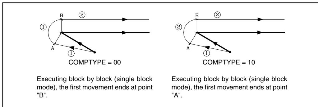
When the beginning or the end of the compensation takes place in a different plane (there is an intermediate vertical movement) and with angle greater than 270°, one should be analyze the CNC's behavior as shown next:
