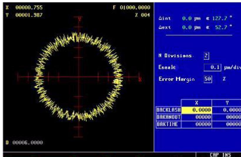
If the machine parameters are protected, it will request the access password because the bottom right of the screen shows some of them. When not knowing the password, those values cannot be changed, but it will be possible to access the screen and the circle geometry test.
