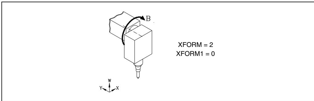
The swinging spindle head "XFORM=2" does not have a secondary or "dragged" axis but parameter "XFORM1" is defined like in the case of the 45° and spherical one.
