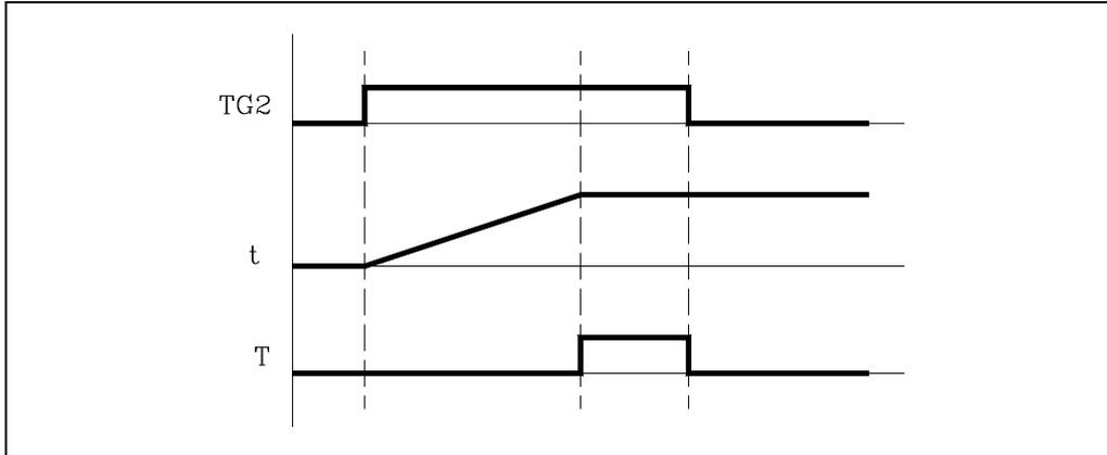
If the timer is initialized with values T<sub>EN</sub>=1 and TR<sub>S</sub>=0, the timer will be activated when a leading edge is produced at TG2 input. At that instant, the timing "t" begins from "0".
