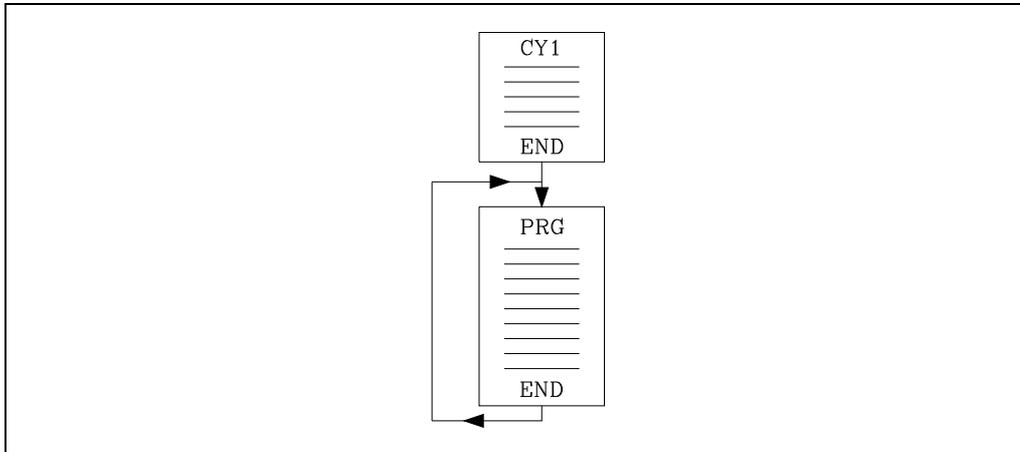
The periodic module will be executed every time the time indicated in the directing instruction "PE t" elapses. This count starts when the execution of the main module (the first time) begins.
