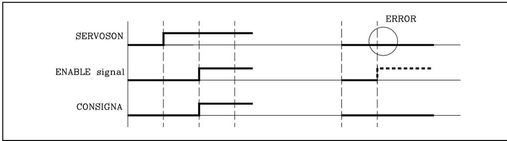
On the other hand, if the SERVOSON signal is low or if it changes to low during the rotation of the spindle, the CNC will stop the axes feed and the spindle rotation displaying the corresponding error message.
