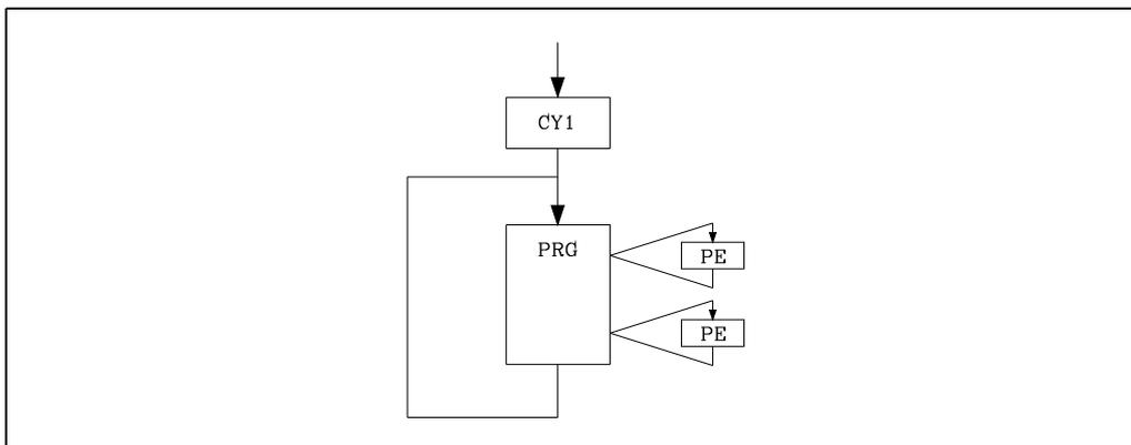
When defining the PLC program, both the processing of the main module (PRG) and the periodic modules (PE) must be taken into consideration.
