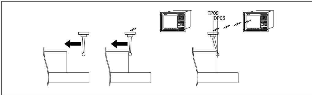
Although the probe keeps moving until the CNC receives the probing signal, the CNC takes into account the value assigned to general machine parameter PRODEL and provides the following information in the variables TPOS(X-C) and DPOS(X-C).
