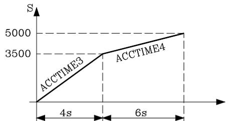
Maximum synch speed: 5000 rpm.
