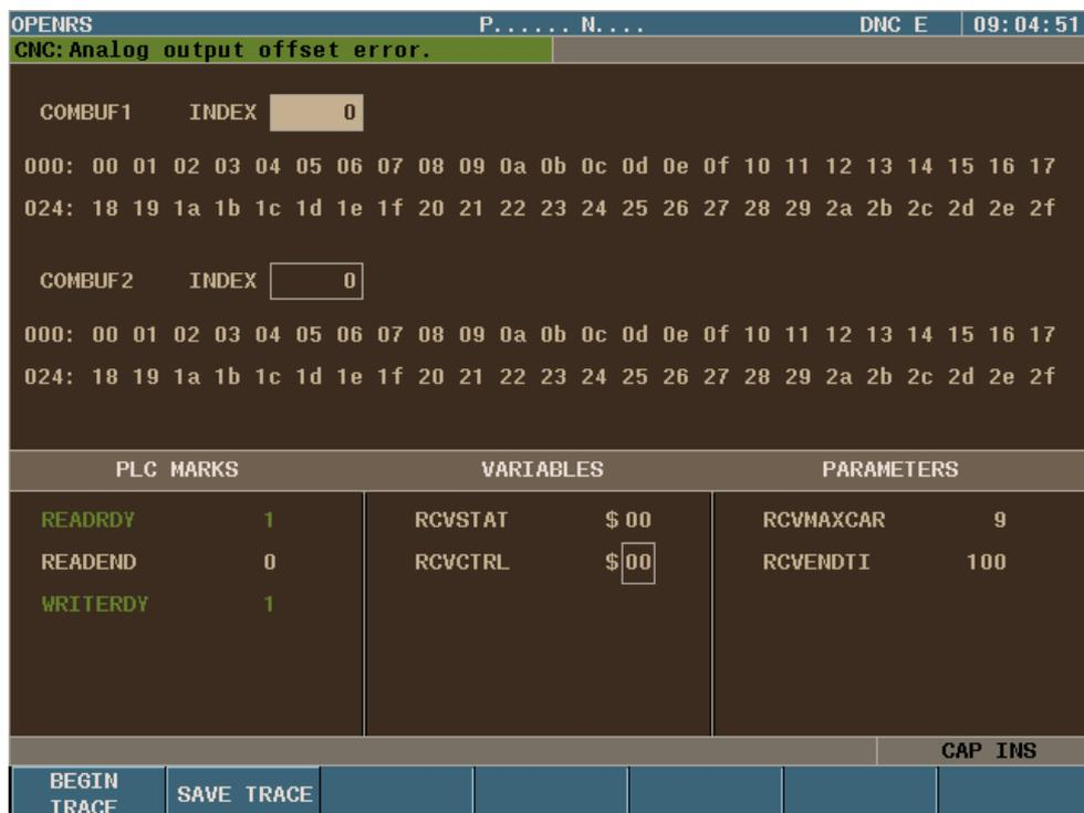
PLC instructions are used to begin a trace, the [SAVE TRACE] softkey must be pressed to save the trace into the KeyCF.
