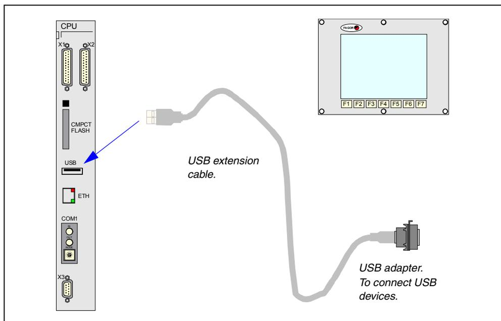
3. Once properly connected to the extension set, the USB devices may be connected through the adapter.
