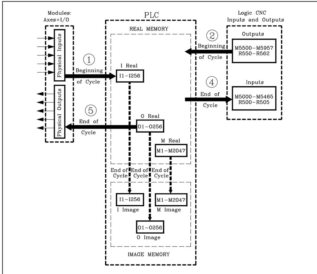
The following example shows how the PLC acts when working with real or image values.
