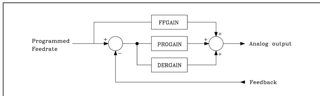
When it is due to variations of the programmed feedrate, "ACFGAIN" (P42) = YES, it is called AC-forward gain" since it is due to acc./dec.
