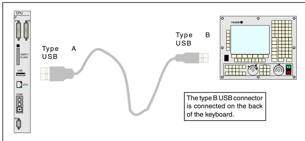
2. Once the extension cable has been properly connected, the USB connector of the keyboard may be used.
