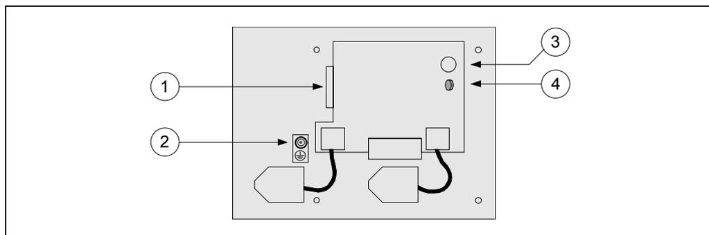
1. SUB-D type 25-pin female connector to connect the keyboard with the central unit or with a switching board.
