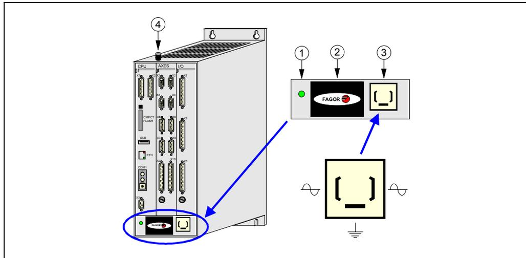
1. Indicator led. When ON, it indicates that the central unit is under power.
