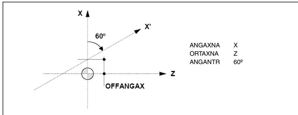
The axes defined in parameters "ANGAXNA" and "ORTAXNA" must exist and must be linear. These axes may have associated with them Gantry axes, coupled axes or axes synchronized by PLC.
