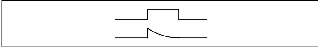
If the duration of the rectangular pulse is adjusted for low speed, it may be too high for high speed or not enough for low speed when adjusted for high speed. In these cases, it is recommended to use the exponential type that applies a strong pulse initially and decreases in time.
