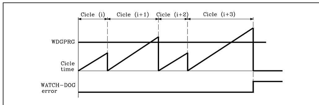
This way, the execution of cycles that, due to their duration, disturb the operation of the machine can be prevented and the PLC can be prevented from executing a cycle which has no end due to a programming error.
