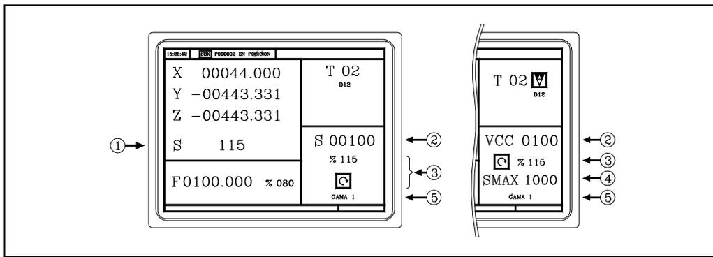
1. Real spindle speed in rpm.
