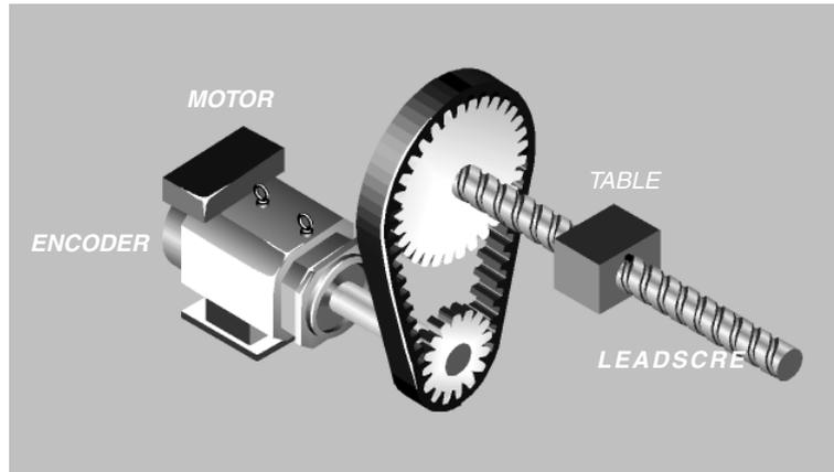
We have an axis with a maximum feedrate of 20 m/min, with a leadscrew pitch of 20 and a 3-to-1 gear ratio between the motor and the leadscrew. The motor encoder provides 2500 pulses per turn.
