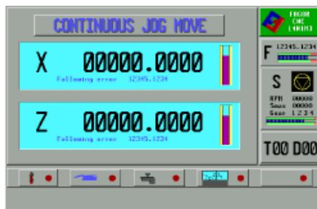
All of them use OEM screens that have been created on a PC using the Fagor WINDRAW55 application software and have been sent out to the CNC using the Fagor WinDNC application software.
