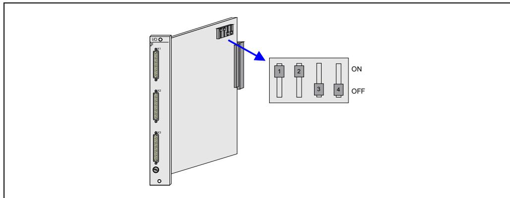
The logic address is set in binary code between 1 and 14. Logic address "0" and "15" are reserved. Logic addresses 0 and 15 are reserved.
