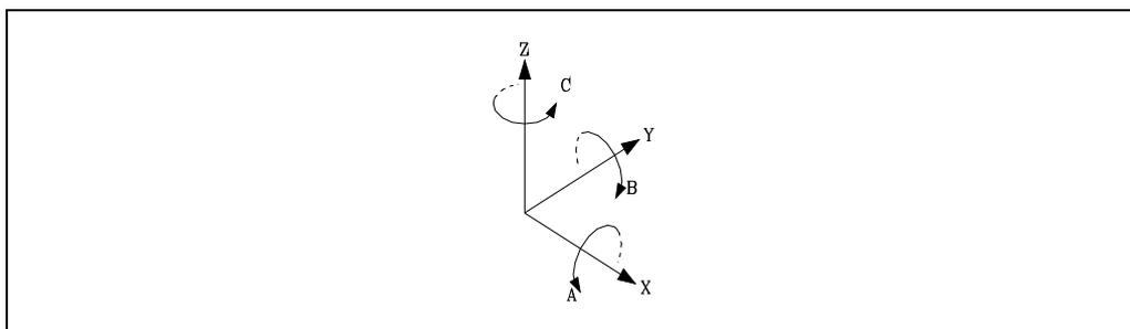
The rotary axes are called A, B or C depending on whether the rotation axis is X, Y or Z respectively. The turning direction of the axes may be changed with parameter "XFORM2".
