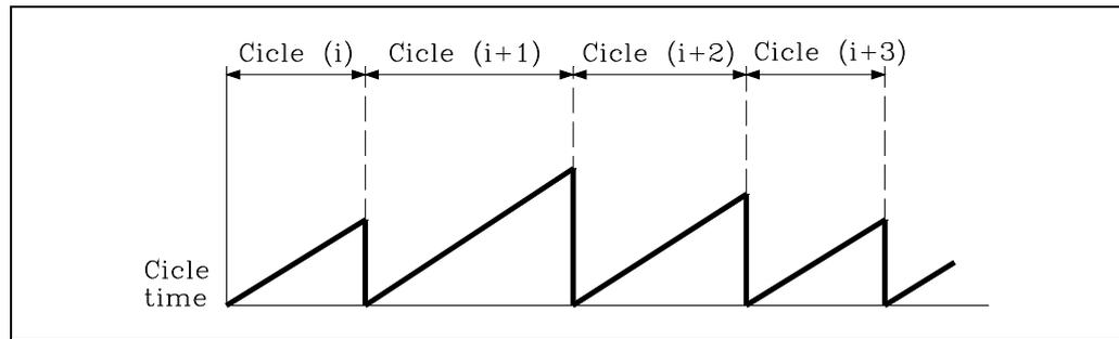
plc.m.p WDGPRG (P0) sets the maximum cycle execution time This is called WATCH-DOG time and if a cycle is executed which lasts longer than 1.5 times this time, or two cycles are executed, one after the other, taking longer than this time period, the CNC will display the WATCH-DOG error of the main module.
