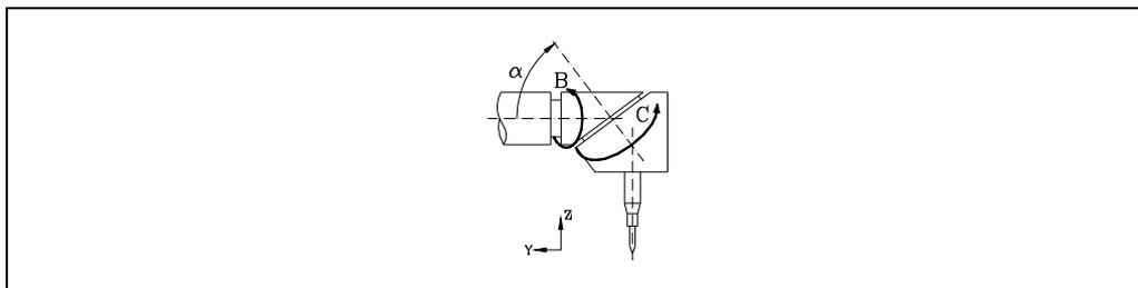
In an angular spindle, the main axis must be parallel to one of the axes X, Y, Z and the secondary axis will be at an angle with respect to it.
