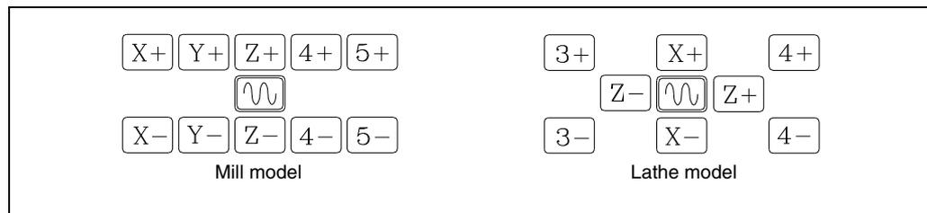
The X, Y and Z axes always use their own denomination; the "C" axis of a lathe model uses the [3+] and [3-] keys and the rest of the axes depend on the chosen name.
