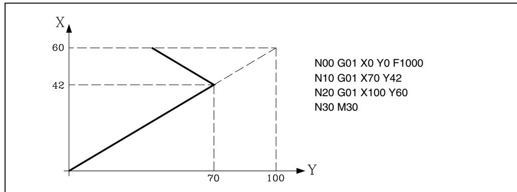
If, when executing the programmed movement in block N20 the signal corresponding to the X axis "MIRROR1" is active, the CNC will apply mirror image to the remaining movement in X.
