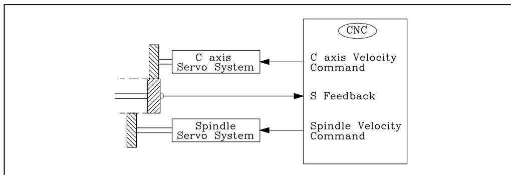
The feedback must be connected to the spindle (S) connector.
