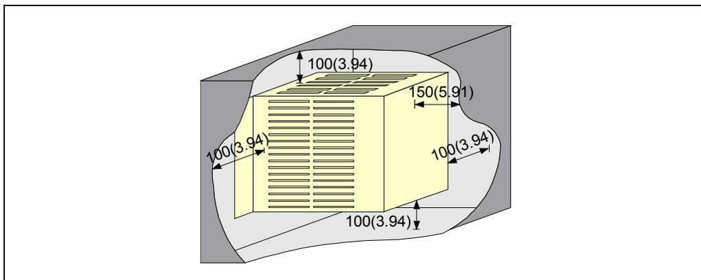
When using a fan to better ventilate the enclosure, a DC FAN must be used since an AC fan may generate electromagnetic interference resulting in distorted images being displayed by the CRT.
