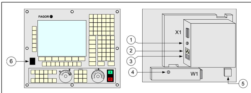
W1 SUB-D type 25-pin female connector to connect the keyboard signals.
