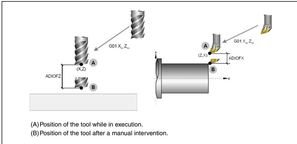
The intervention with an additive handwheel is only possible in execution mode, even while the program is interrupted. However, it is not allowed in the tool inspection mode.
