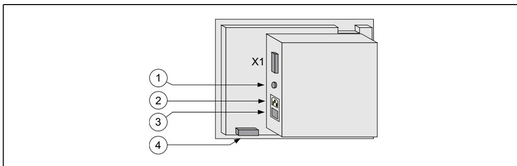
X1 SUB-D type 25-pin male connector to connect the video signals with the central unit.
