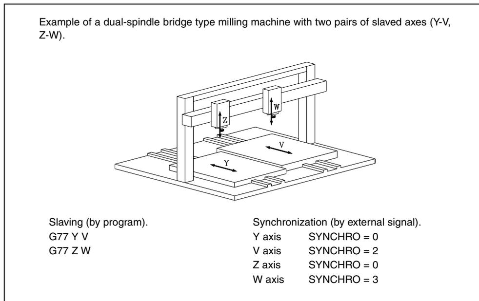
If the machine has the X, Y, Z, V, W axes, the following signals must be activated (logic state "1") at the PLC:
