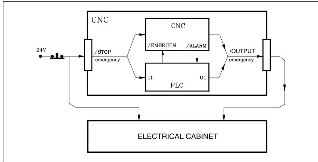
When the PLC sets the "/EMERGEN" input low (0V), the CNC stops the axes and the spindle and it displays the corresponding error message.
