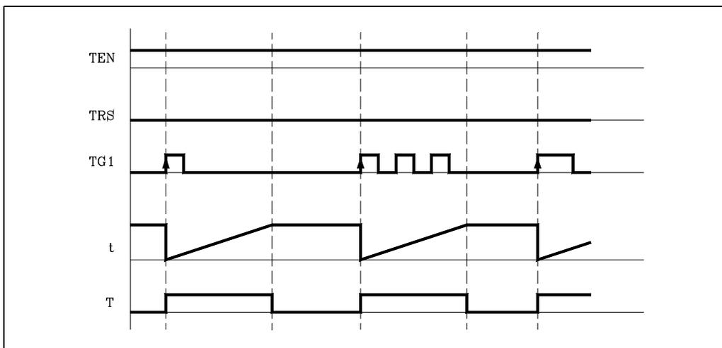
Once the time specified by the time constant has elapsed, timing will be considered as having finished. The timer status output (T) changes status (T=0) and the elapsed time will be maintained with the time value of the timer (T).
