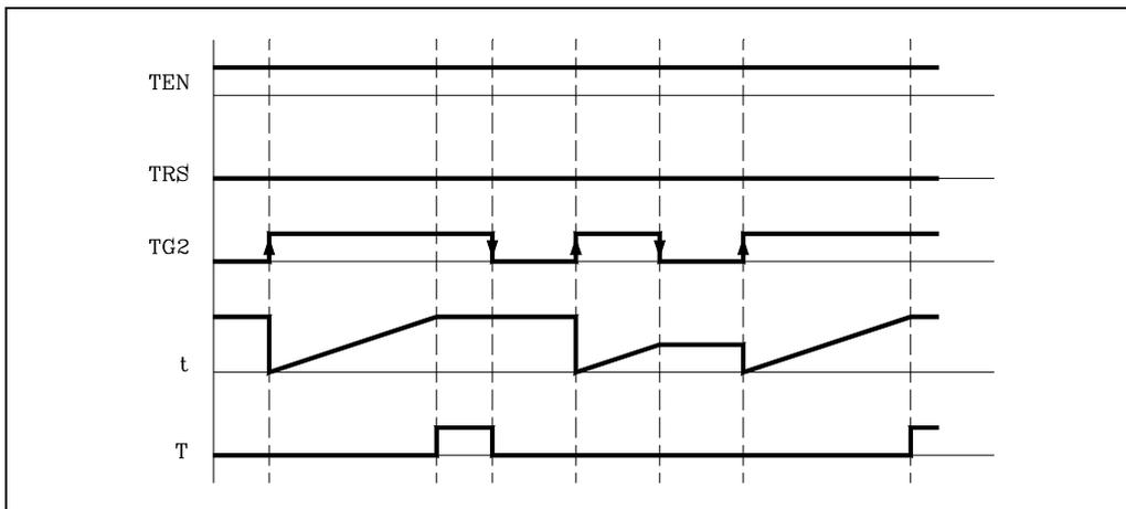
If, once the timing has finished, it is required to activate the timer again, another leading edge must be produced in the TG2 input.
