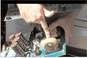
Ron points to an induction coil that gets hotter than 250 °F. He can frequently troubleshoot these boards by using a heat sensor that can indicate whether or not the component is working. No heat (a cold heat sink) can indicate that an item like a transistor is not working.
