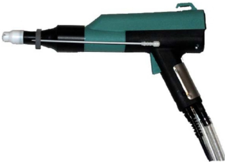
Illustration 8 An MG801 with a low ion adaptor
