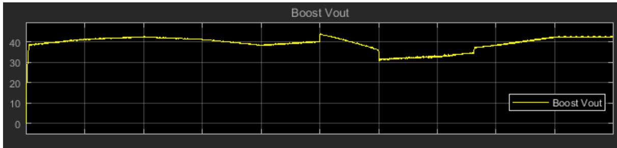
Fig.8 Boost Voltage from the solar panel
