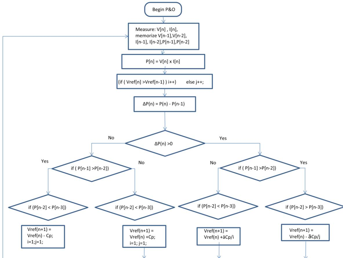
Fig.6 Perturb and Observation Algorithm
