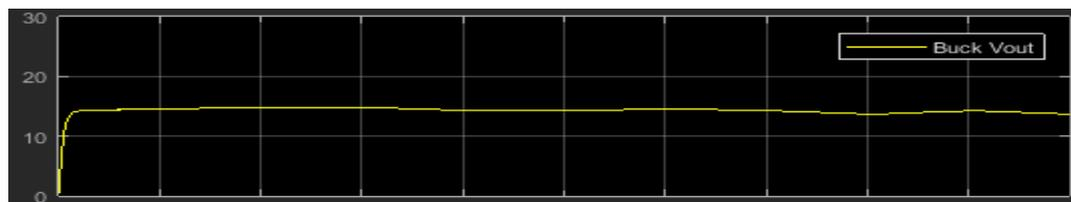
Fig.14 Output voltage from buck converter
