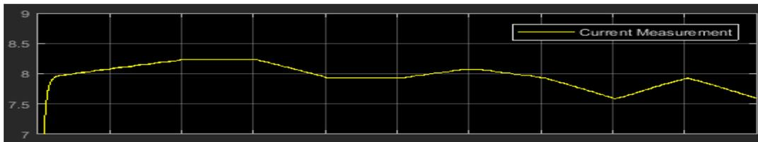
Fig.15 Output current from buck converter
