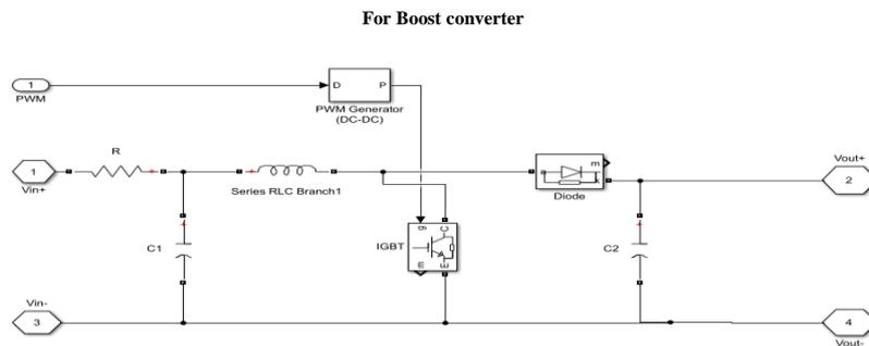
Fig. 4 Simulation model for the DC-DC boost converter
