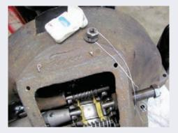
Tie the washer and nut on the string of dental floss in order as they will go onto the shaft. It is easy to turn the nut several threads onto the pedal shaft until you can feel the end of the shaft just protruding from the nut.
