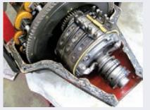
Another nylon tie strap may be used to tie the clutch release ring fork to the clutch lever shaft. Tying the ring prevents it from dangling and flopping as the hogshead is lowered over the crank-
