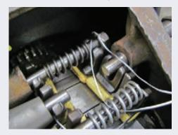
Now break away the dental floss. Any remains are just teflon and won't cause trouble. Place the floss-tied spring on the low speed pedal shaft and fit the low speed adjustment screw.
