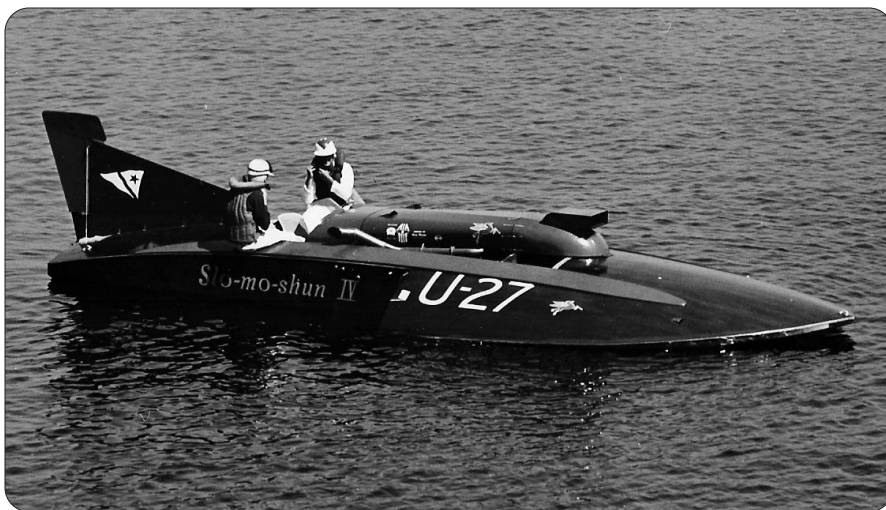
The Grand Old Lady with its set-up for the 1952 straightaway record attempt. An air scoop has been added to the nose cowling.
