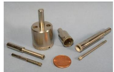
Chuck the core drill in a drill press, Dremel or Foredom and be sure to keep the drilling zone wet to cool the tool and to flush out debris. Also, if you're drilling a through hole, go very easy on the pressure as the drill is about to cut through. Otherwise you will usually chip off some of the stone surface around the hole.
