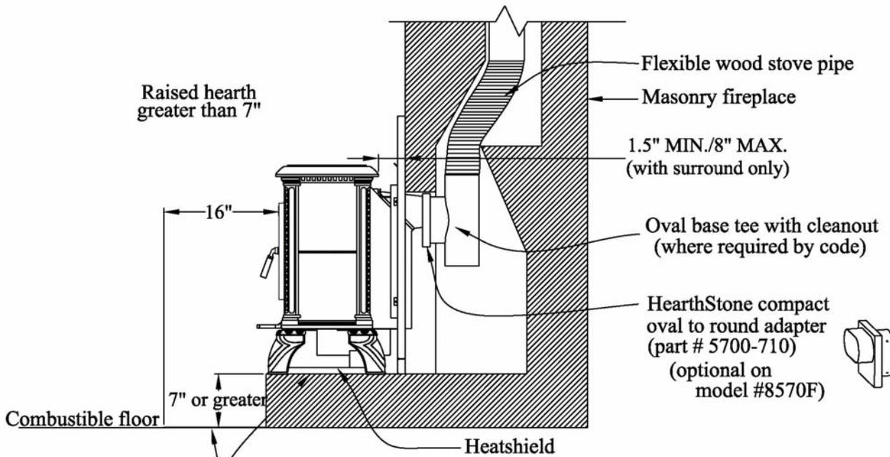
Floor protector beneath the stove and extending 16" in front of glass and 8" beyond either side of the fuel and ash door openings
