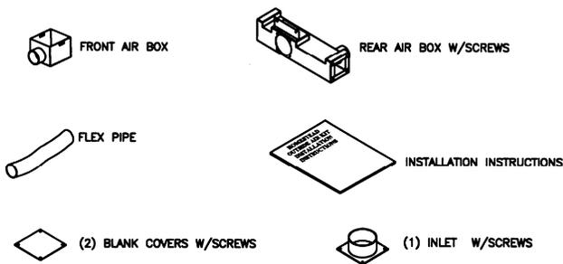
The Outside Air Kit allows for a direct stove connection of a 3” (76 mm) diameter duct (which you can obtain from another manufacturer); this duct leads to the outside of the house. Connect the duct to your stove in a number of ways (illustration is typical for both Hearth Mount and Freestanding models). Choose the one that is most convenient.
