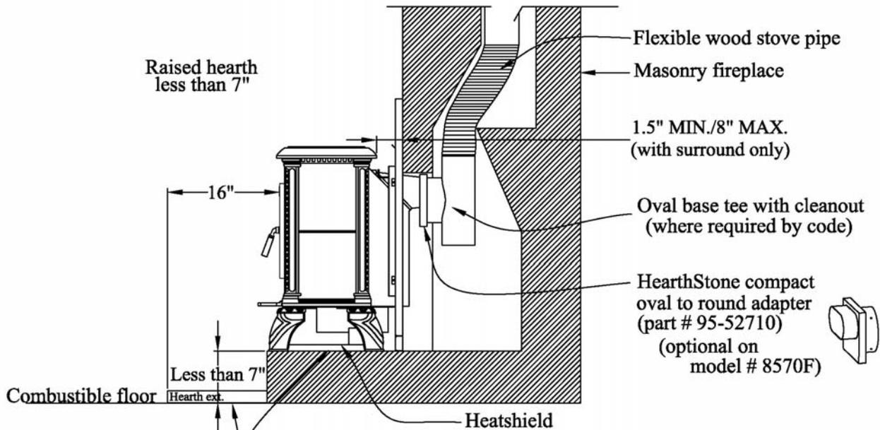
Floor protector beneath the stove and a hearth extension with an "R"-value of 2.5 or listed to U.L. 1618, extending 16" in front of glass and 8" beyond either side of the fuel and ash door openings.
