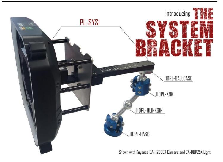
A simple way to mount the newest Keyence Multi-Dimensional Vision System CA-DQP25X with a camera all on one setup. This System Bracket, **PL-SYS1** gives you a 10 inch range to mount your camera above the light. It is made up on anodized aluminum, stainless steel mounting plate with stainless steel fastens. The PL-SYS1 is only compatible with our HDPL Series. Hardware for the HDPL-BALLBASE is included, but the HDPL-BALLBASE is not included.
