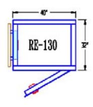
Right hinge door swing shown. Left hinge door swing available. Window placement always on wall opposite hinge. Indicate model number and door swing at time of order placement.
