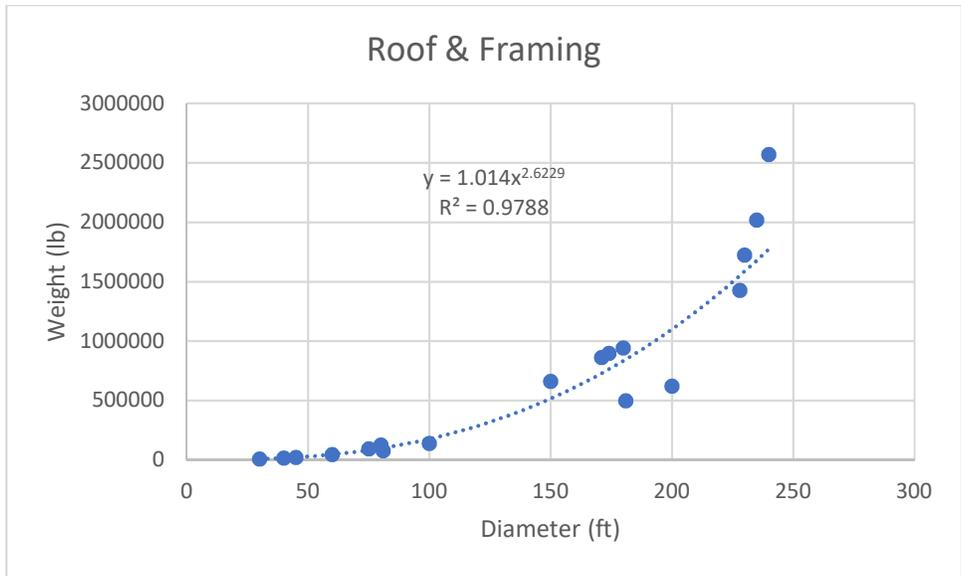
Figure 2 - Roof and Framing Weight Estimation for Fixed Cone Roofs
