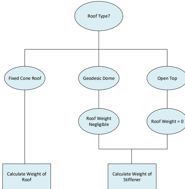
Figure 1 - Flow Chart of Roof Weight Calculation
