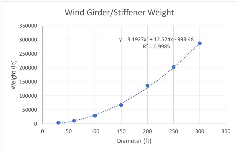
Figure 3 - Stiffener Weight Estimation
