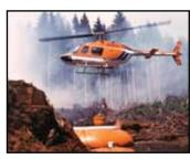
**Helitanks** are designed for water delivery to ground crews in areas with steep slopes and limited water resources. The Helitank can be secured by a sling around a tree or stump and attached to two large 'D' rings on the uphill side. Specifically designed for Type 2 helicopters, Helitanks are available in two sizes.
