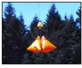
Effective on remote, steep, sloped terrain, the **Stilwell Flyer** is transportable by helicopter with long line delivery. The tetrahedron shape of the Stilwell Flyer eliminates twisting and residual bounce in flight. The Stilwell Flyer ensures safe and reliable transport of water to crews in remote locations.
