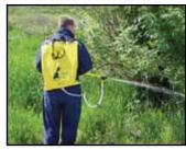
The **FlexPak** was one of the first lightweight collapsible water backpacks used by fire fighters for site mop-up. In addition to its collapsible backpack tank, the FlexPak includes a hand pump for fire control which can be equipped with a reservoir for foam concentrate application.
