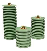
Epoxy Mica Couplers (EMCs) are permanent sensors used to detect PD activity while not affecting the operation of the machine. These are used to only allow high frequency (>40Mhz) signals to pass through, collected and analyzed.
