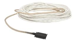
The Flux Probe is a non metallic sensor installed within the stator that detects the magnetic field emanated from each rotor pole. This is used to determine if there is a presence and the severity of failures.
