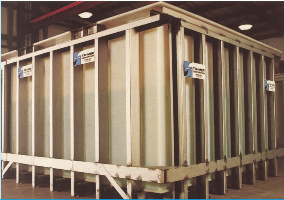
Completed 10' wide x 12' long x 8' deep H 2 SO 4 pickling tank constructed of 1" thick polypropylene with 316L stainless steel cradle support.
