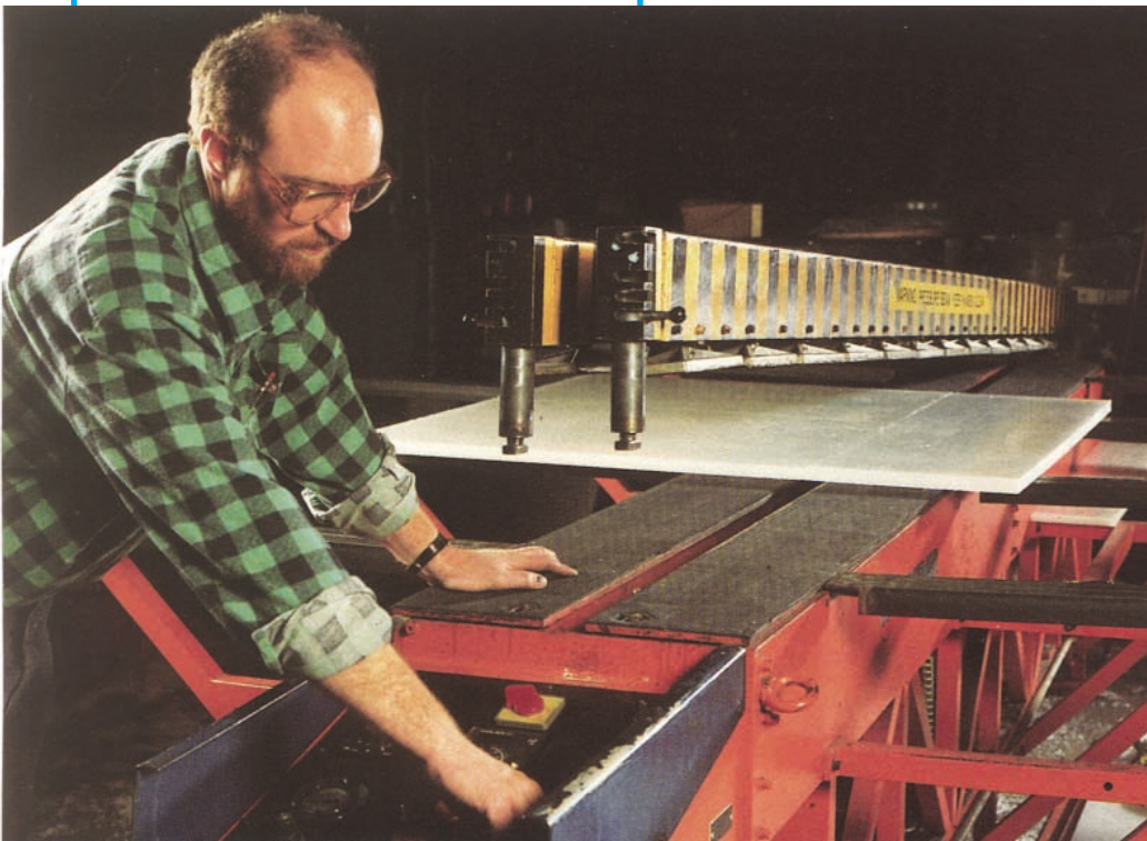
Automatic welding machine joining flat sheet polypropylene
