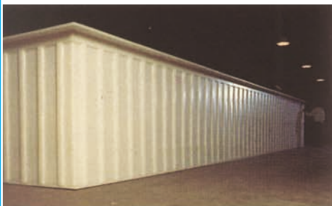
Fully fabricated 45' long tank ready for exterior support structure
