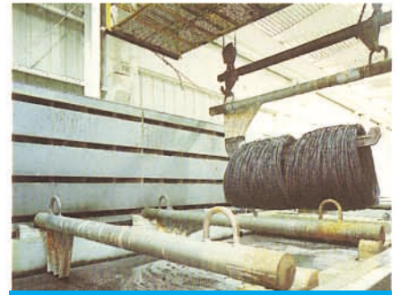
H 2 SO 4 pickling tanks in operation.
