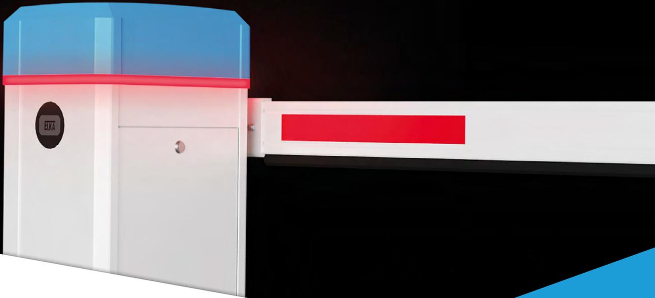
The transparent plastic ring with LED strips is integrated between the barrier housing and hood and evenly illuminated in all directions (red / green / blue or warm white selectable). The type of lighting (permanently luminous or flashing) is freely configurable via the controller MO 24. The visibility of the barrier system is significantly increased in darkness and in poor visibility conditions.
