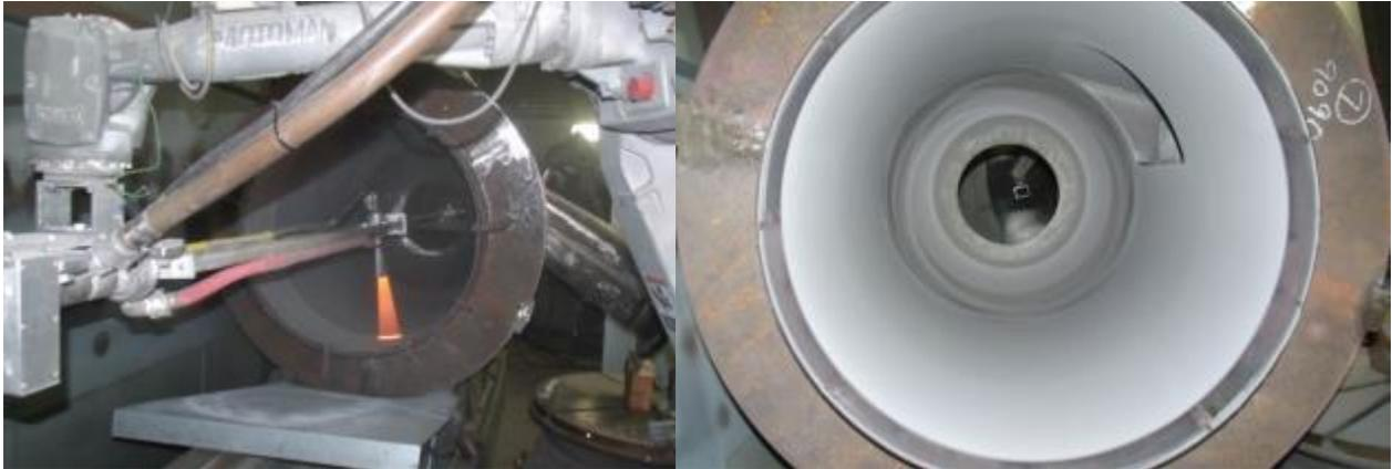
The WC-10Co-4Cr coating applied in the refinery coke transport line cyclone with rotating AK-5 gun. The cyclone was 33-inch diameter, 5-feet long. The 4-foot protruding transition nozzle did not allow the cyclone rotation. The rotating shaft supported the further end of the gun, making available liner movement up to 6 feet.
