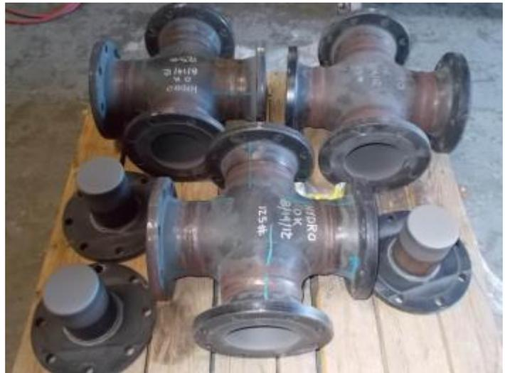
Application of WC-10Co-4Cr coating with rotating AK-ID gun inside the elbows, 6" (150 mm) ID:
