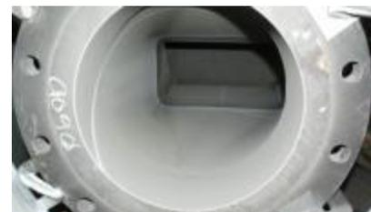
Application of WC-10Co-4Cr coating with rotating AK-5 gun inside the double-elbow of a coke transport line. The elbow internal diameter 12 inches, total length 6 feet.
