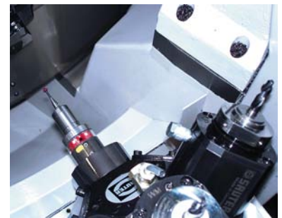
Fast workpiece measurement in rotary transfer machine
