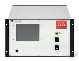
The ModBox-DER is the first equipment specially designed to measure the Dynamic Extinction Ratio (DER) of high contrast ns optical pulses in the 1000 nm wavelength band. It measures Extinction Ratios up to more than 50 dB, for pulses as short as 5 ns, from single-shot operation to 10 kHz repetition frequency.
