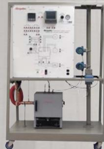
**MODEL H-ICS-TT** Hampden Instrumentation and Controls Temperature Process Loop Trainer
