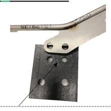
STEP 1 LOCATE MOUNTING HOLES IN CLOSING FRAME.
