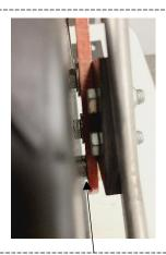
STEP 3 Install 3/8" bolts and tighten. Repeat for other side.
