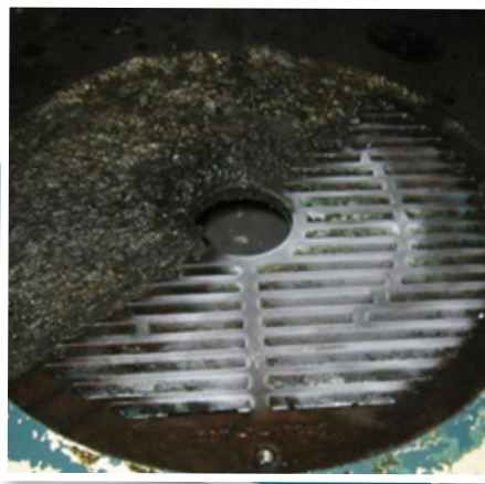
Cold Jet dry ice cleaning was used to remove the surface contamination on a fan cover at an automotive manufacturer in Michigan. After implementing regular cleaning with dry ice, there was an instant energy savings of 42% for the company.
