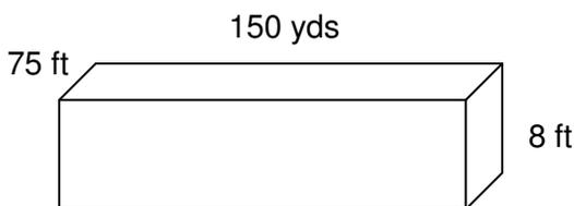
When we multiply feet X feet X feet, our answer is given in CUBIC FEET – therefore, if we do our volume according to the formula of surface area X average depth, our answer will be in cubic feet. However, in pools, we refer to the volume of water in GALLONS. So, once we do our surface area X depth calculation, we have to convert cubic feet to gallons. Since each cubic foot can hold approximately 7.5 gallons of water, the complete volume formula is: Surface area X depth X 7.5 = gallons.
