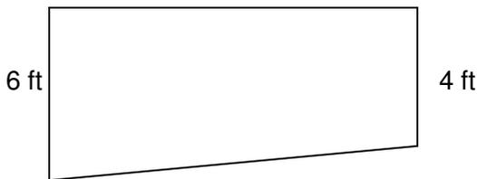
Sometimes, we need to determine the AVERAGE DEPTH of a pool with a sloped bottom. To calculate the average depth, we do a simple 'average' calculation; Add the shallow depth + the deep depth, and then divide by 2. This formula will work only if the pool bottom has a constant slope – one angle from shallow to deep, as pictured here.
