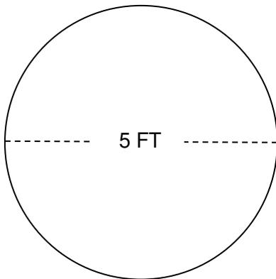
A Sand Filter has a Diameter of 5 ft and has a filter media rate of 10 gallons per minute per sq ft of filter area. What is the maximum flow rate this sand filter can handle?
