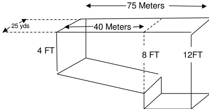
When calculating volume (gallons) for a pool with multiple depths, it is best to break the pool into multiple components based off of those depths
