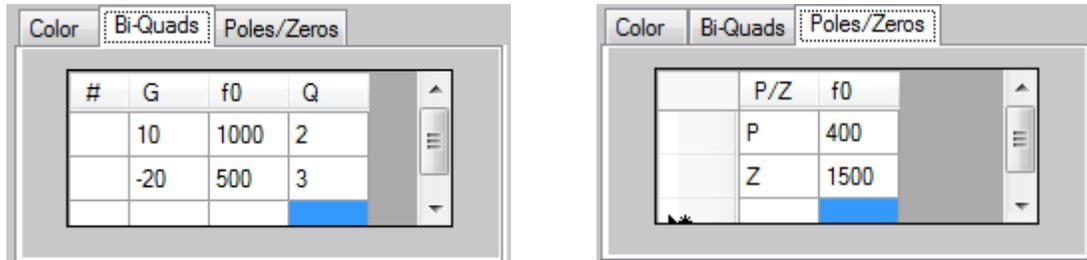
These parameters were applied to white noise with an 18dB/Octave HPF at 40Hz and a 36dB/Octave LPF at 15 kHz to yield this result.
