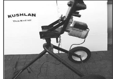
**Step 5.** Install Gear Box Frame with 5/8" x 10" Pivot Pin.
